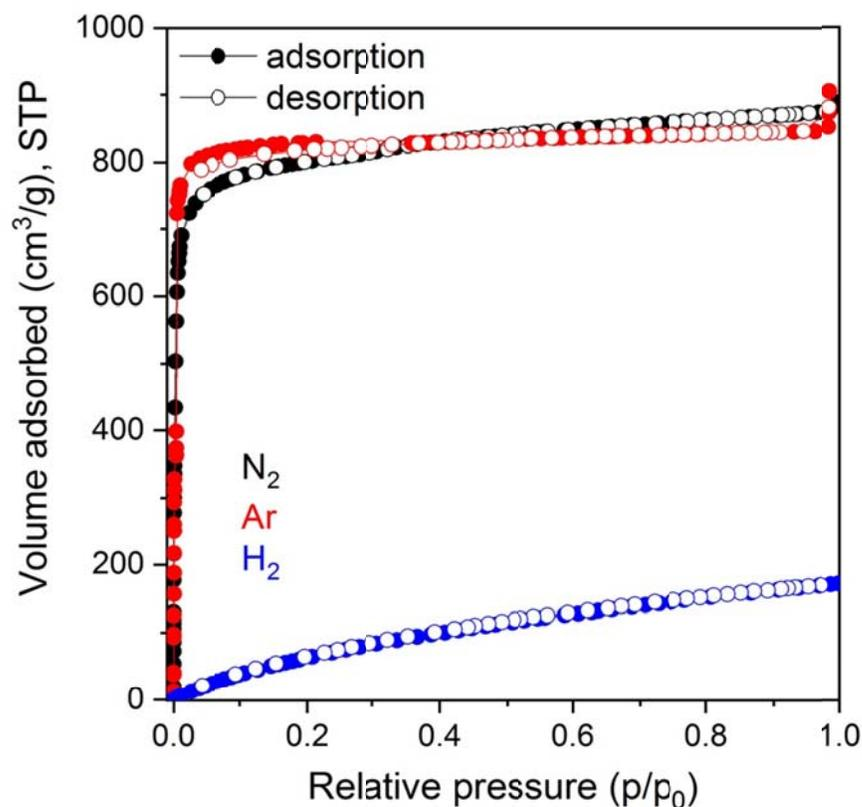
**Figure 5.** Adsorption isotherms of basic zinc cubane-dicarboxylate, **1**.
