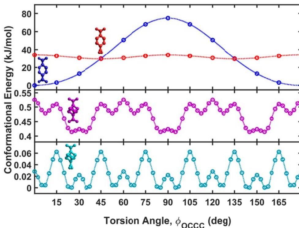
**Figure 4.** Calculated conformational energy of various fragments of basic Zn-1,4-dicarboxylate and MOF-5. a:  $D_{2d}$ -dicarboxylate of **1**, b:  $D_{2h}$ -dicarboxylate of **1**, c: blue:  $D_{2h}$ -dicarboxylate of MOF-5, red: hypothetical  $D_{2d}$ -dicarboxylate of MOF-5.
