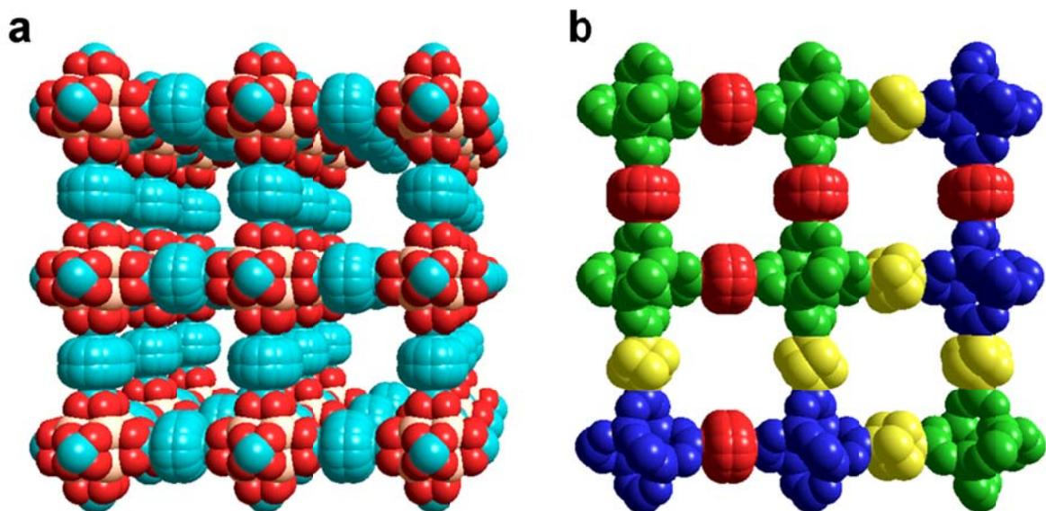
**Figure 2.** Perspective view of the crystal lattice of basic zinc cubane-1,4-dicarboxylate, **1**. a: Average structure, corresponding to the  $Pm\bar{3}m$  space group. b: A snapshot of the (001) plane between the temperatures of the predicted 2-step freezing of the spacers. An orientational glass of two perpendicular SBUs (green and blue) are connected with static (yellow) and rotating (red) cubylene units.
