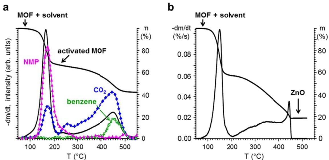
**Figure 1.** Thermal decomposition of **1** (a) in inert and (b) oxidative atmospheres. Solid lines: TG and DTG curves,  $-\blacktriangle-$ , NMP ( $m/z$  99),  $-\diamond-$ ,  $\text{CO}_2$  ( $m/z$  44);  $-\square-$ , benzene ( $m/z$  78);.
