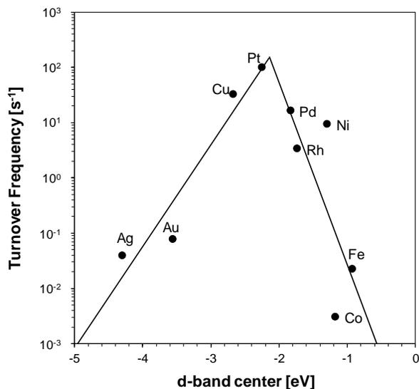
**Figure 1. Experimentally measured turnover frequency of vapor phase formic acid decomposition to CO and CO<sub>2</sub><sup>12</sup> as a function of the metal d-band center.<sup>13</sup> Turnover frequencies were measured at steady state in a packed bed reactor at 523 K and 2000 ppm formic acid in He with < 2% conversion.**
