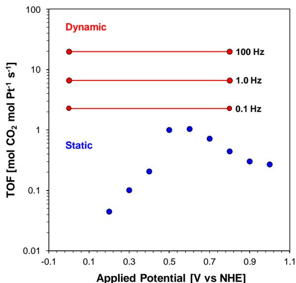
**Figure 9. Comparison of Dynamic and Static Electro-catalytic Oxidation of Formic Acid on Pt.** Static formation rate of CO<sub>2</sub> from formic acid (blue) at fixed applied potentials ( $0.2 \leq V \leq 1.0$ ) is significantly lower than the dynamic turnover frequencies (red) varying at 0.1, 1, and 100 Hz with square waveforms at 50% duty cycle with an amplitude of zero to 0.8 V applied potential.
