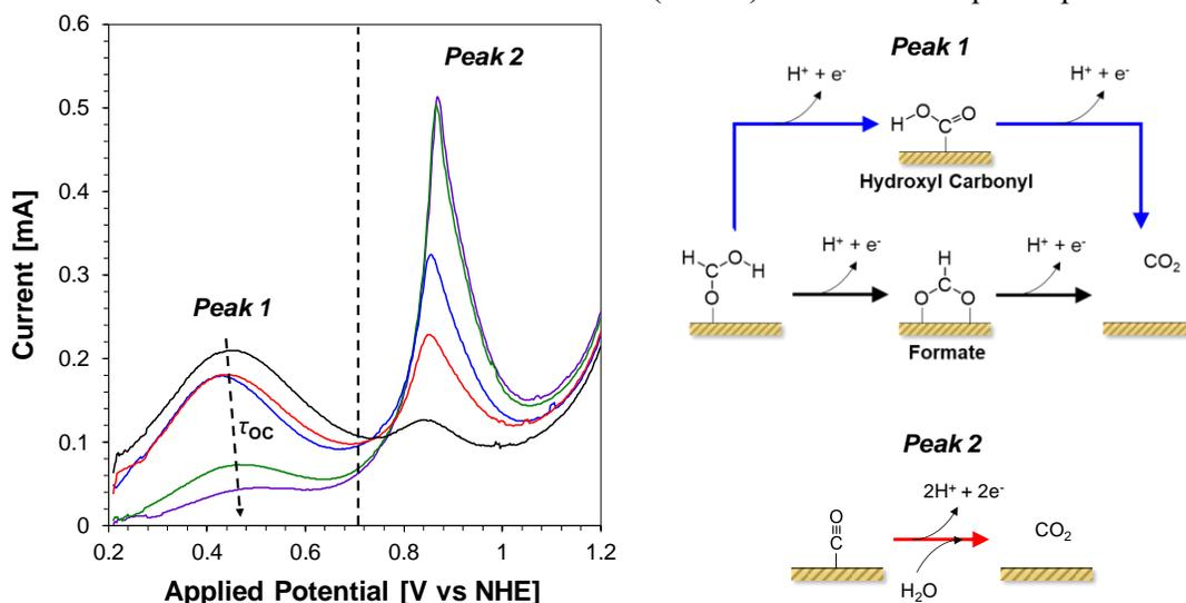
**Figure 7.** Linear sweep potential curves ( $100 \text{ mV s}^{-1}$  scan rate) with varying initial hold times at open circuit ( $\tau_{\text{oc}}$ ). Two peaks are associated with direct electro-oxidation (peak 1) and  $\text{CO}^*$  oxidation (peak 2).
