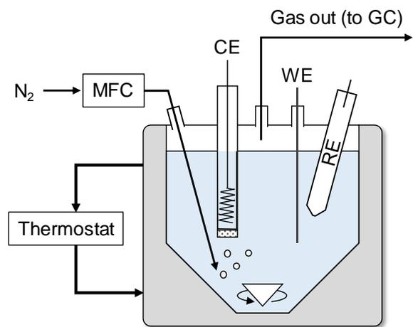
**Figure 3. Electrochemical cell with continuous gas flow and online gas chromatography analysis.** MFC – Mass flow controller, CE – Counter Electrode, WE – Working electrode, RE – Reference electrode, and GC – Gas Chromatograph.
