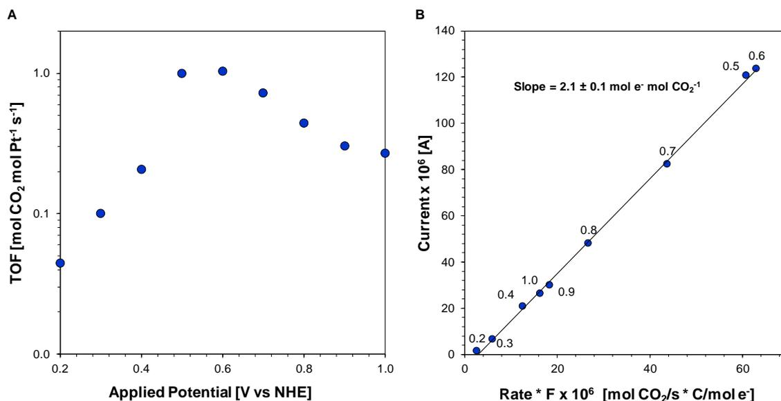
**Figure 4. Polarization Curve: Steady-State Formic Acid Electro-oxidation on Pt.** (A) The turnover frequency of formic acid electro-oxidation was determined at steady state on Pt by measuring the continuous rate of carbon dioxide formation with online gas chromatography as a function of applied potential. (B) Measured current as a function of the rate of reaction multiplied by Faraday's constant at various applied potentials, error in slope estimated at 95% confidence interval.
