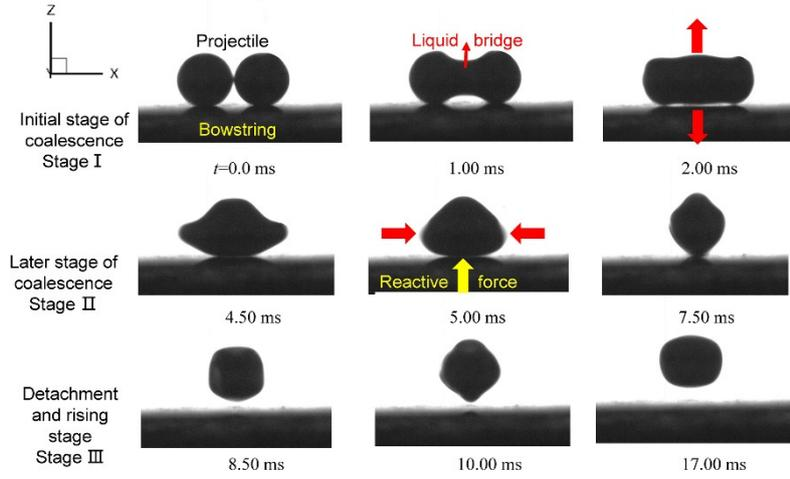
Fig. 1. The morphology evolution of liquid metal droplet with time in case 1. The volume of a single droplet is  $2.5 \mu\text{l}$ , and the radius is  $842 \mu\text{m}$ . The velocity of the droplets when they depart the surface is about  $0.160 \text{ m/s}$ . Two groups of red arrows in the figure respectively indicate the expansion of the liquid bridge and the contraction of the droplets.
