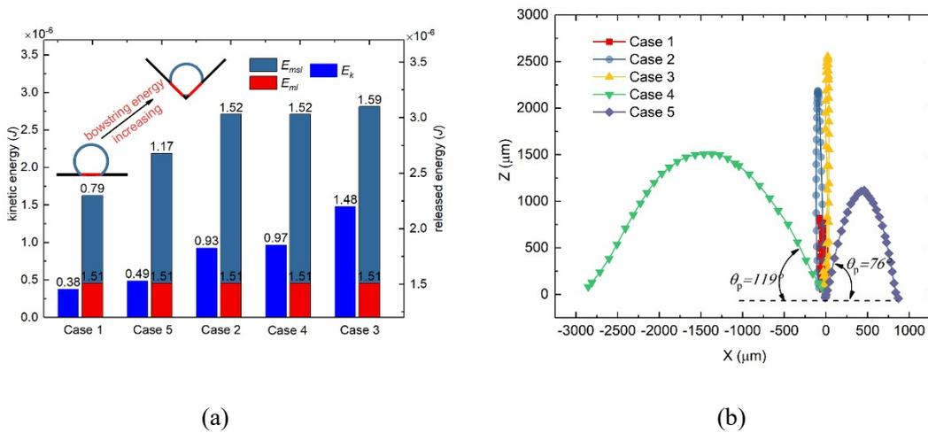
Fig. 5. (a) The relationship between projection kinetic energy, bowstring energy, and bowstring shape. The calculation of kinetic energy takes the average projection velocity of three experiments for each case. (b) The relationship between the projection direction and the shape of the bowstring. Case 1 is the case shown in Fig. 1. The radii of droplets are  $842 \mu\text{m}$  in all cases and the substrate
