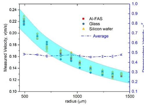
Fig. 3. Change of projection velocity and dimensionless velocity with droplet radius
