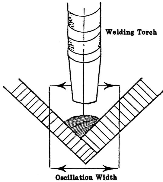
Fig. 5. *Through the arc sensing system with an oscillating torch.*
