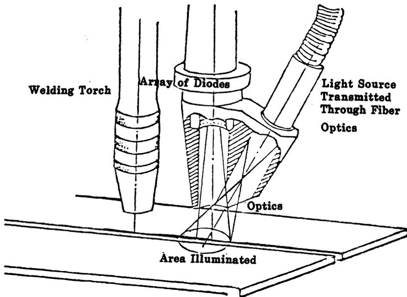
Fig. 2. Joint characterization by linear array of photodiodes.
