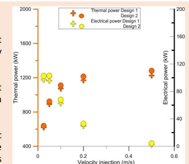
Figure 6: Thermal and Electrical power produced at 10 years using an Organic Rankine Cycle power plant.
