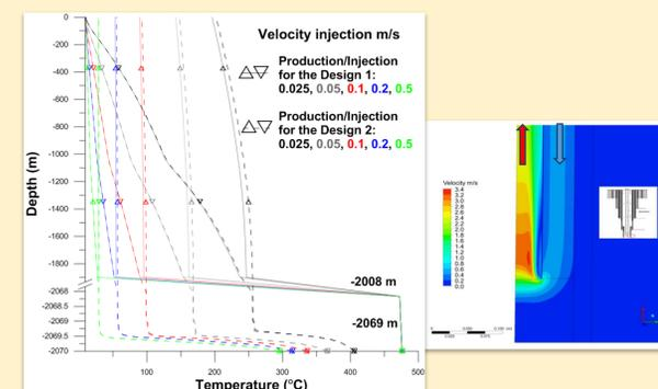
Figure 4: Left - Vertical temperature distribution after 10 years in both injection and production wells for the two designs. Right - Velocity distribution in the bottom hole around -2069 m for Design 2.
