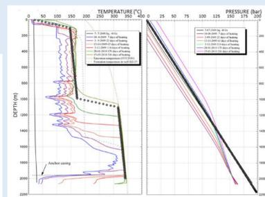
Figure 2: Temperature and Pressure initial conditions compared to data measured in the IDDP-1 (up to 2km).
