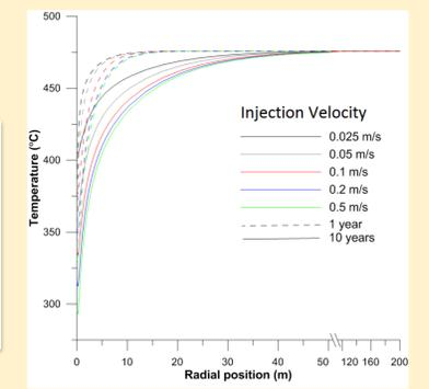
Figure 5: Radial-Temperature distribution at -2070 m for the Design 2 at 1 and 10 years
