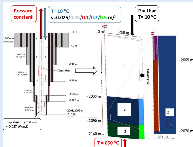
Figure 1: Left - Full Weissbad DBHE description and simulated domain (red dashed-lines), modified from Kohl et al. 2000. Right - Axisymmetric DBHE model showing all 3 porous zones, as detailed in Table 1, and boundary conditions. The far right pictures shows a closer view of the bottom hole area for Design 2.
