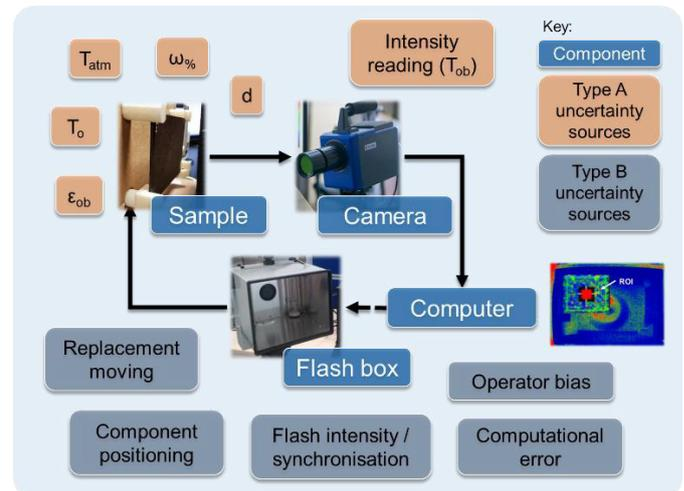
Fig 1. Setup diagram with uncertainty in thermography system
