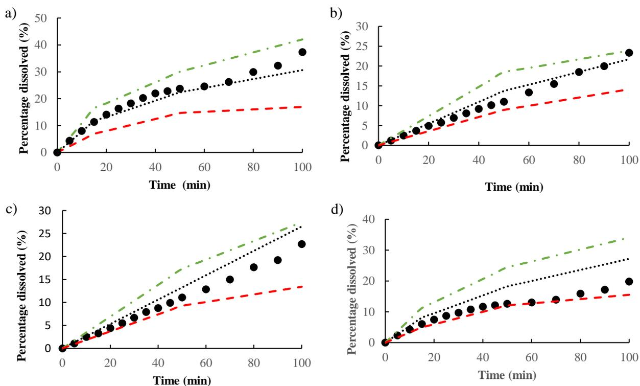
**Figure 6.** Comparison between the GoldSim simulation, including dissolution rates as a distribution element and 101 realizations using Monte Carlo, and laboratory experiment dissolution rate curves for NTQ (a) DNAN (b) RDX (c) and the IHE (d). The dots indicate experimental results and the discontinuous line is the simulated results from GoldSim. Green, red and black discontinuous lines indicate maximum, minimum and mean breakthrough, respectively.
