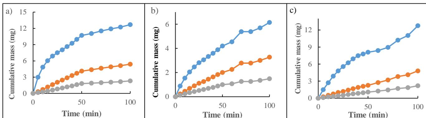
**Figure 5.** Dissolved cumulative mass of the IHE compounds over time of flake A (a), flake B (b) and flake C (c). The lines show NTO (blue), DNAN (orange) and RDX (grey).
