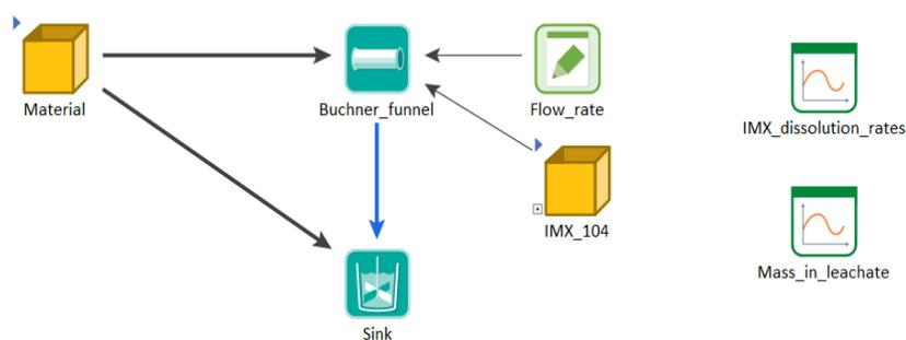
**Figure 2.** GoldSim scheme for the dissolution rate of the IHE formulation
