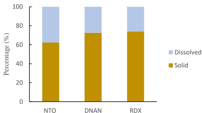
**Figure 4.** Percentage of NTO, DNAN and RDX (average) dissolved (blue) and remaining (khaki) in the flake after the dripping tests.
