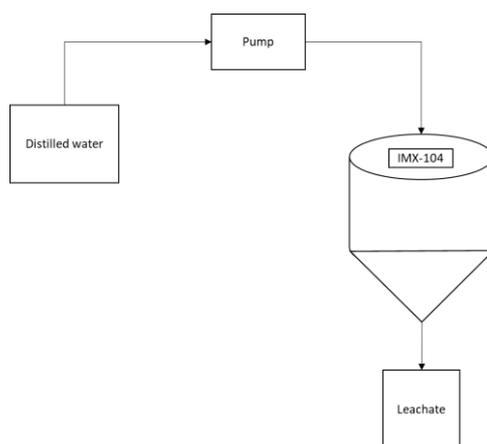
**Figure 1.** Schematic illustration of the experimental setup for the study of the IHE formulation dissolution rate
