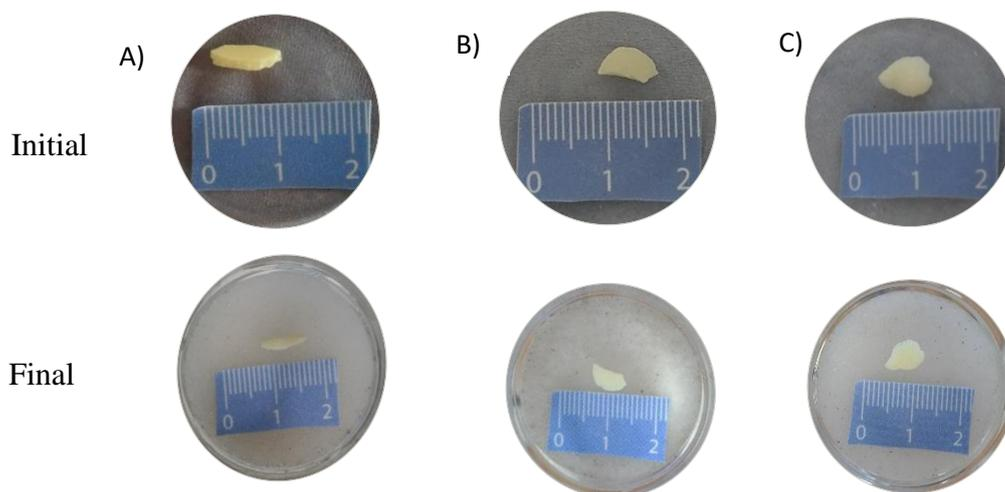
**Figure 3.** Digital photograph of IHE flakes before and after the dripping tests (4L) showing the discolouration and mass loss.
