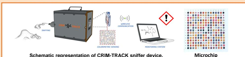
The **CRIM-TRACK** sniffer device includes an air sampling system, colorimetric sensor system, monitoring station and wireless communication between sniffer and monitoring station.
