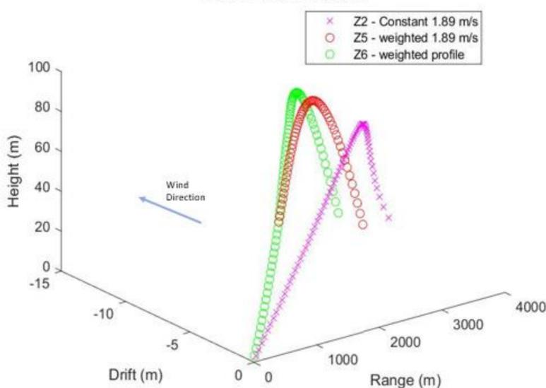
Figure 2 – 3 Axis Trajectory Comparison
