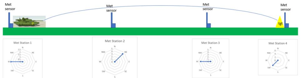
Figure 1 – Range Template Meteorological Wind Station Set up (3)
