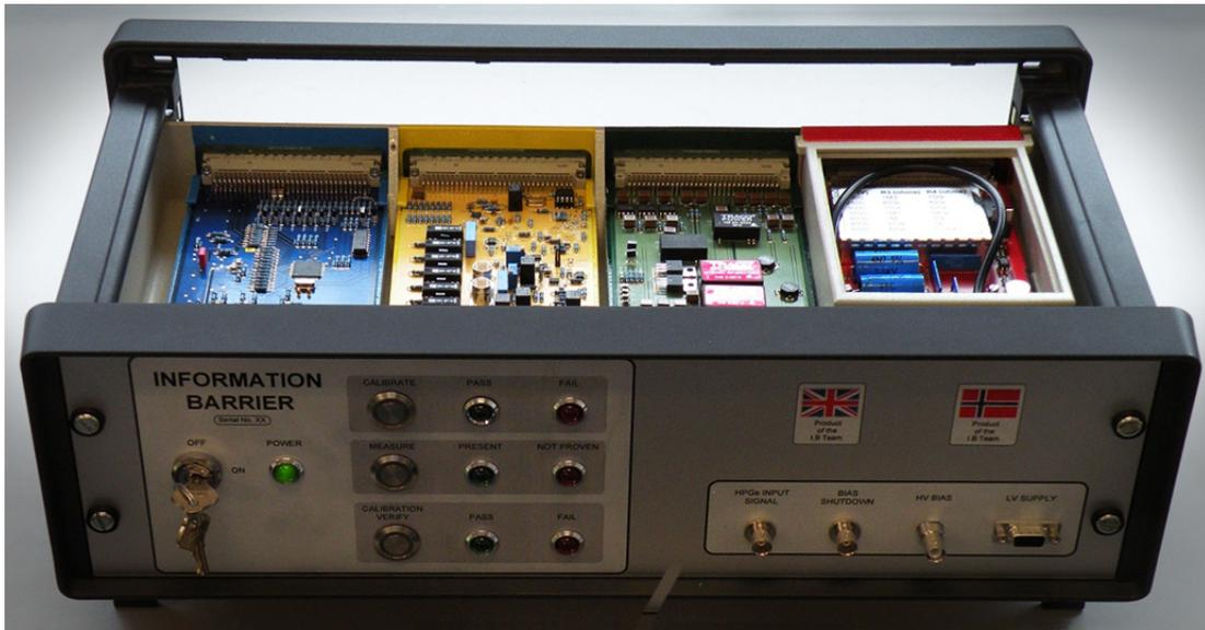
**Fig. 1.** The Information Barrier built as part of the UK-Norway Initiative [13,16]. The option to ‘calibrate’, ‘measure’ and ‘calibrate’ again can be seen on the front of the panel, along with the corresponding (unlit) green and red lights.
