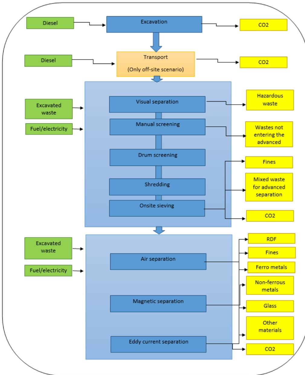
**Figure 3: Process flow diagram of LCA**
