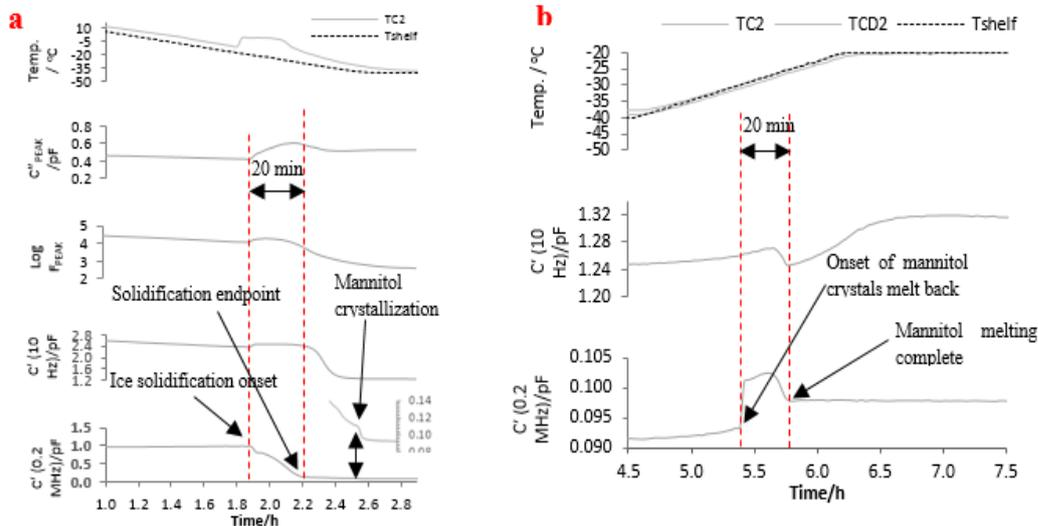
**Fig.1 a)** Shows how  $C''_{PEAK}$ ,  $\log F_{PEAK}$  and Temperature change with time; events that occur with time. **b)** Demonstrates  $C''_{PEAK}$  response to the melting mannitol crystals during re-heating period.
