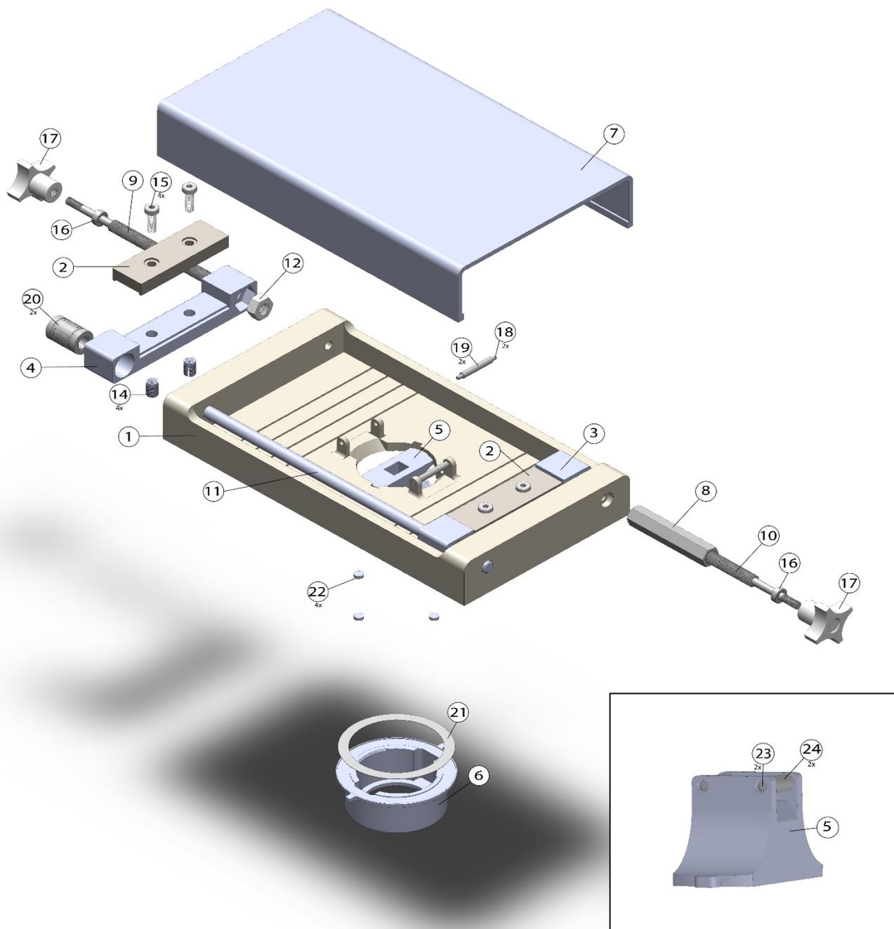
**Figure S2:** Exploded view of the assembled device, with annotation numbers as described in Tables S1 and S2. Since some regions of this device experience high localized stress during tension, the 3-D printed components included structural support features such as side ribs (1) for the base plate and gussets for the indenter (5, in inset).
