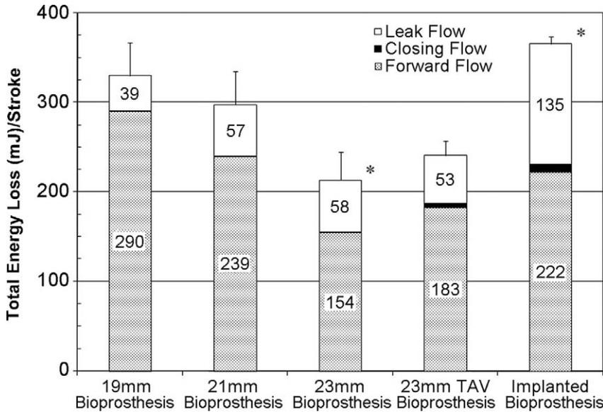
Fig 3. Total energy loss of three Carpentier-Edwards Perimount bioprostheses, and the TAV before and after implantation within the 23mm bioprosthesis. (□ = leak flow; ■ = closing flow; ▨ = forward flow; \* is  $p < 0.001$ .)
