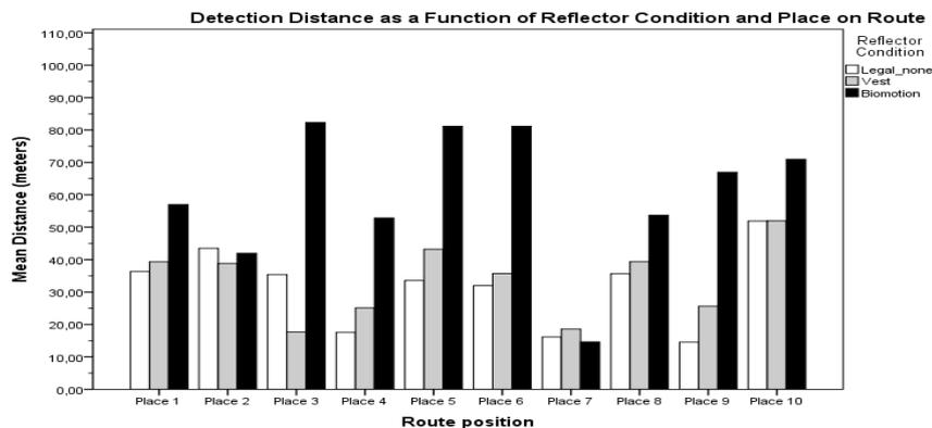
Figure 2: Distance detection in meters as function of reflector condition and place on route.
