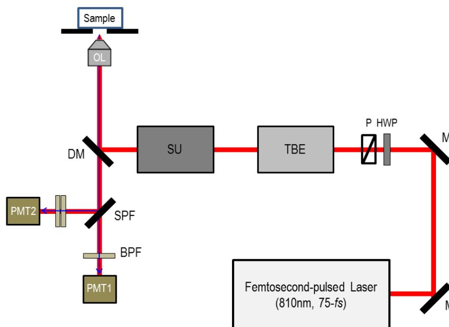
**Fig. S1.** Schematic diagram of optical setup of a nonlinear optical microscopy. Blue arrows indicate backward signals emitted from the samples. HWP: half-wave plate, P: polarizer, TBE: telescope beam expander, SU: scanning unit, OL: objective lens, DM: dichroic mirror, SPF: short-pass filter, BPF: bandpass filter, and PMT: photomultiplier tube.
