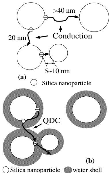
**Figure 12:** Charge carrier movement through overlapping water shells
