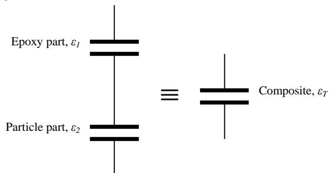
**Figure 14:** Consideration of particle and matrix in series
