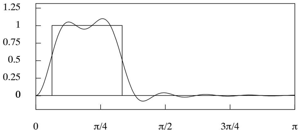
**Figure 4.** The frequency response of a truncated bandpass filter of 25 coefficients superimposed upon the ideal frequency response. The lower cut-off point is at  $\pi/15$  radians ( $11.25^\circ$ ), corresponding to a period of 6 quarters, and the upper cut-off point is at  $\pi/3$  radians ( $60^\circ$ ), corresponding to a period of the 32 quarters.
