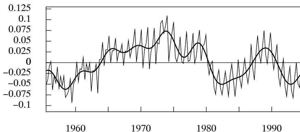
**Figure 9.** The residual sequence from fitting a linear trend to the logarithms of the Gross Domestic Product data. The interpolated line, which represents the business cycle, has been synthesised from the Fourier ordinates in the frequency interval  $[0, \pi/8]$ .
