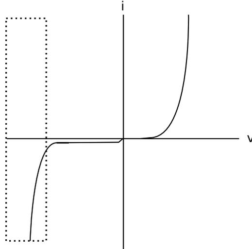
**Figure 1. Voltage current characteristics of a diode (note the negative voltage and current scales are not the same as their respective positive scales).**
