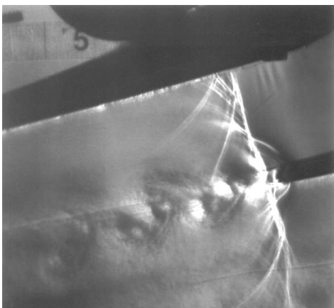
Figure 1: von Kármán vortex shedding at Ma = 0.97
