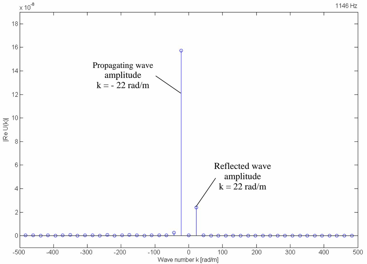
Figure 17. Real part of the wavenumber spectrum of the displacement showing propagating and reflected wave components at 1147 Hz.
