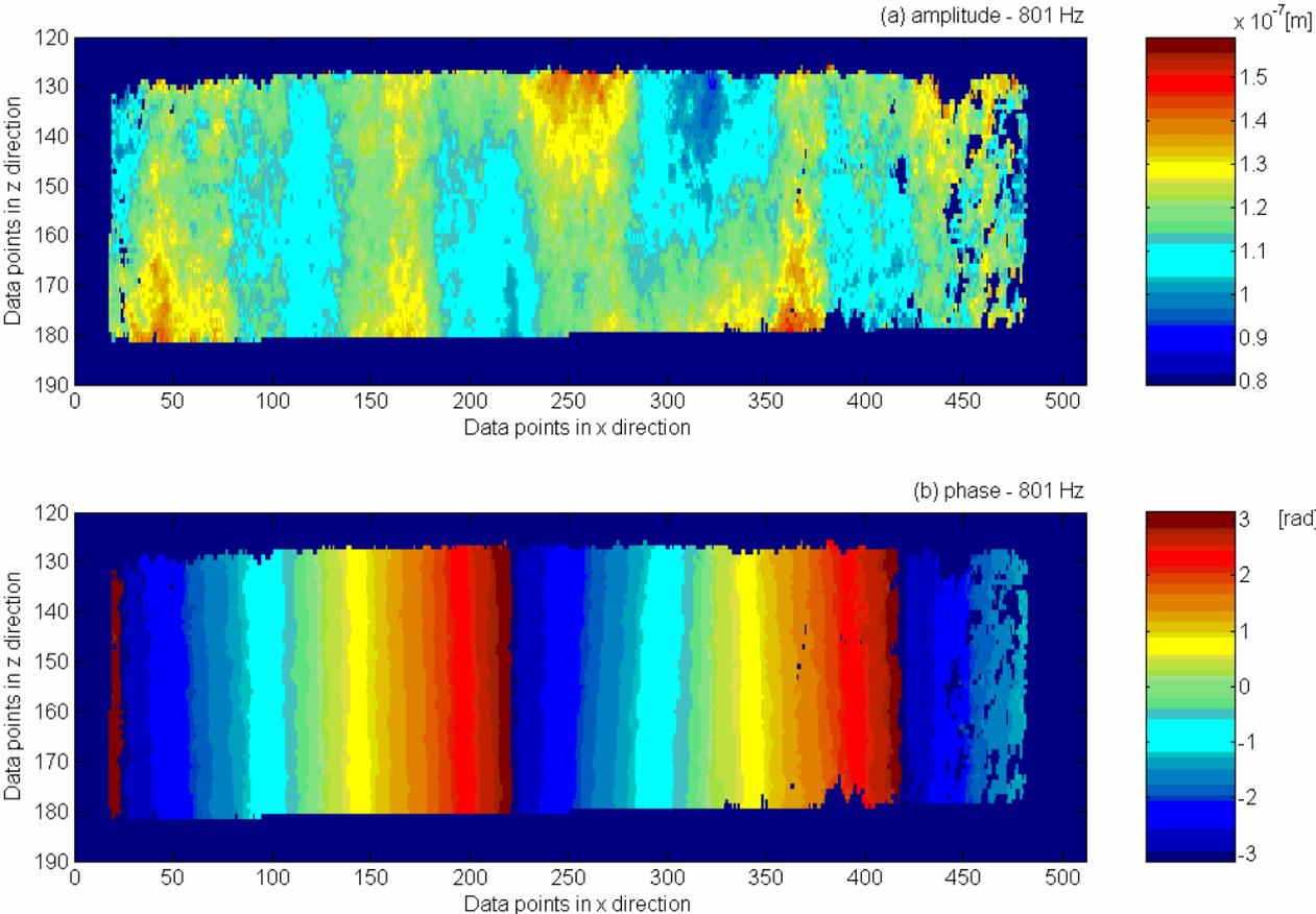
Figure 5. ESPI image of beam displacement excited by a harmonic force at 801 Hz, (a) amplitude, (b) phase.
