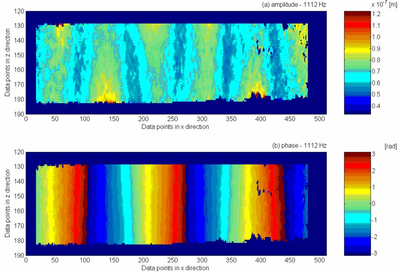
Figure 6. ESPI image of beam displacement excited by a harmonic force at 1112 Hz, (a) amplitude, (b) phase.
