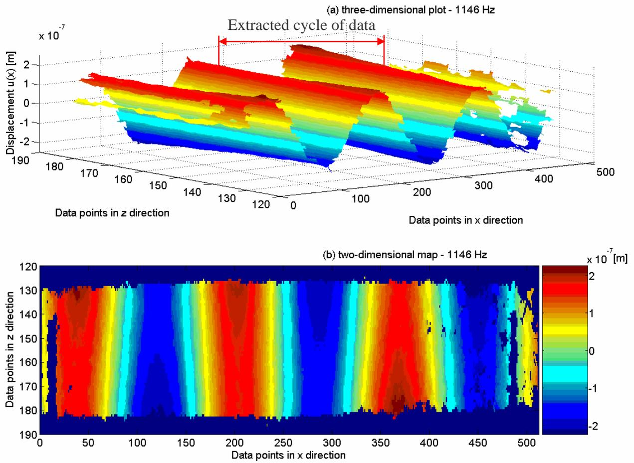
Figure 11. Real part of the beam displacement at 1146 Hz showing the single cycle extracted for wavenumber transformation: (a) three-dimensional plot, (b) two-dimensional map.
