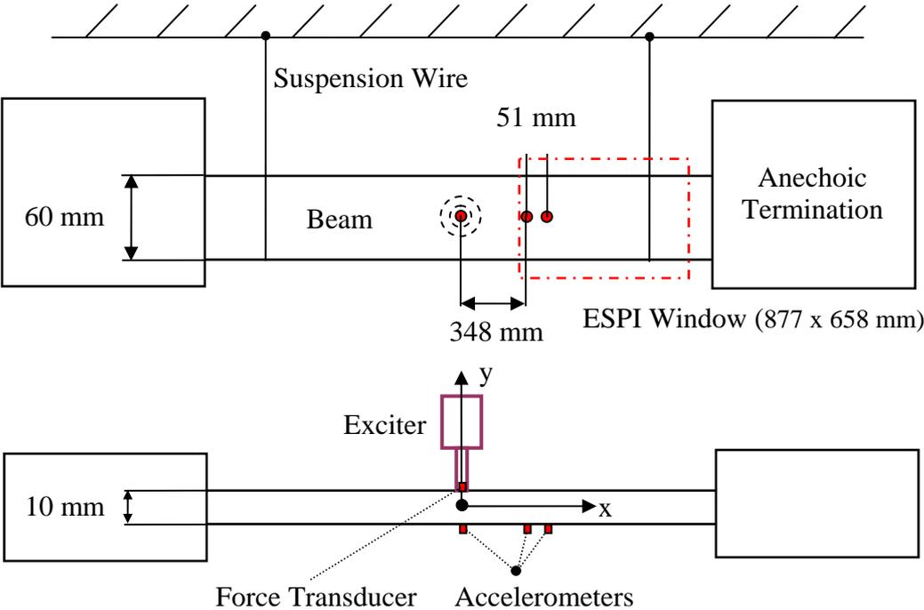
Figure 1. Experimental "infinite" beam apparatus.
