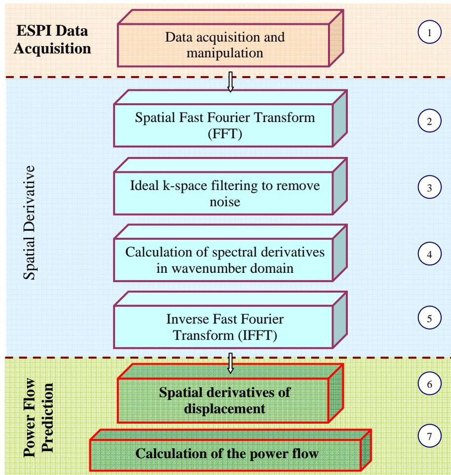
Figure 3. Flow diagram of power flow calculation.
