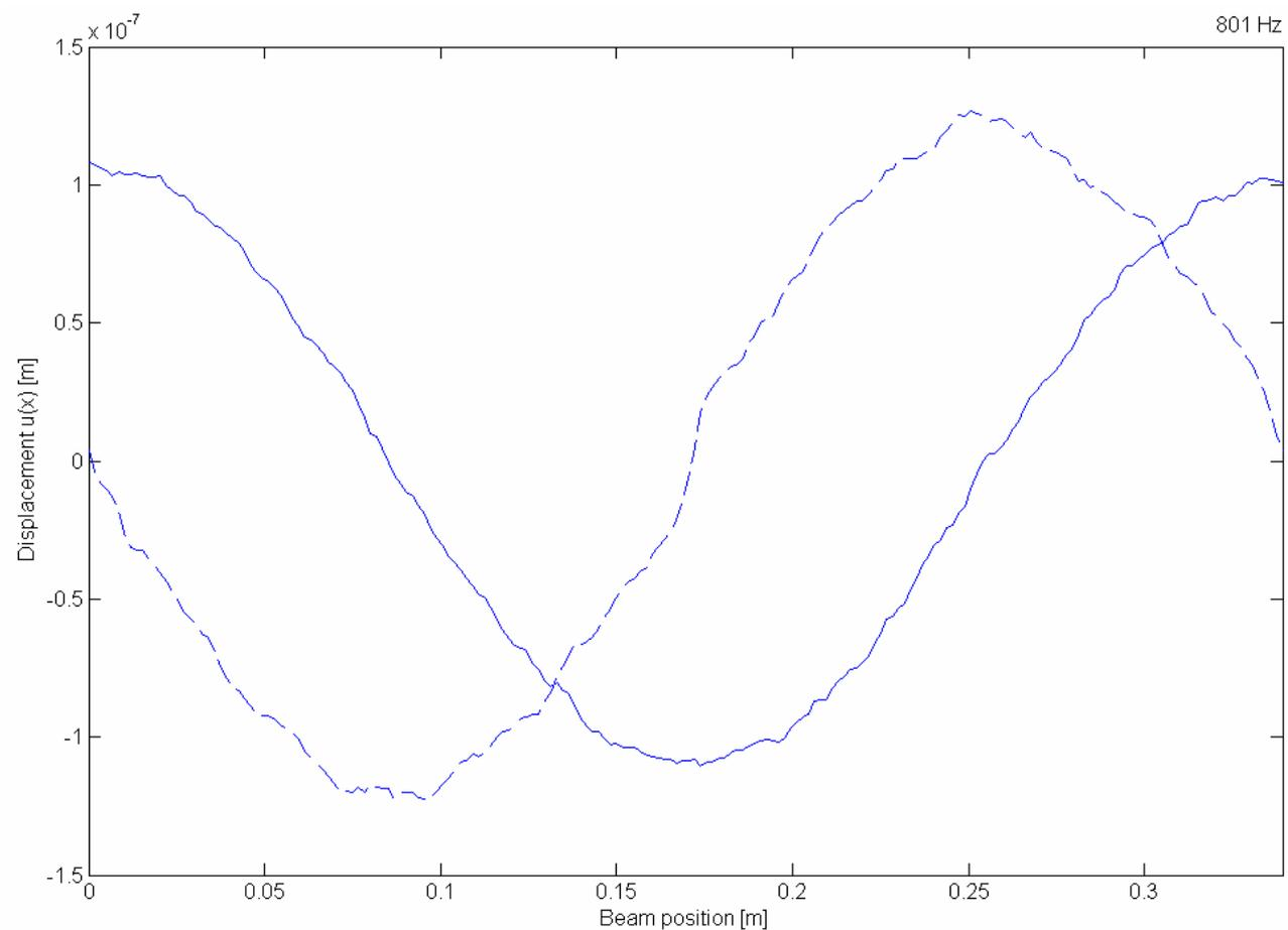
Figure 12. Real part (—) and imaginary part (----) of row 150 from a single cycle of beam displacement at 801 Hz.
