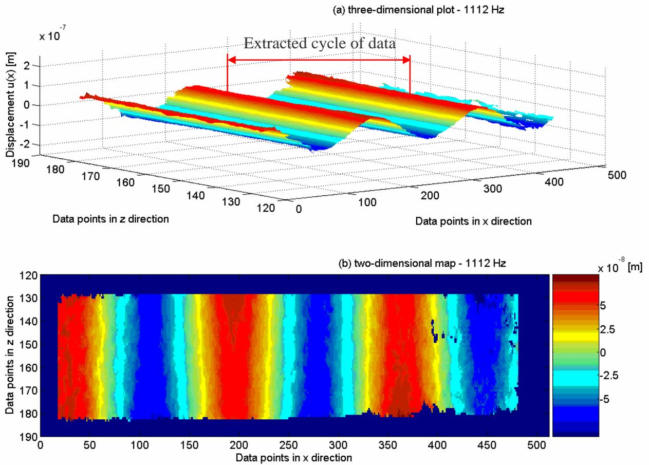
Figure 10. Real part of the beam displacement at 1112 Hz showing the single cycle extracted for wavenumber transformation: (a) three-dimensional plot, (b) two-dimensional map.
