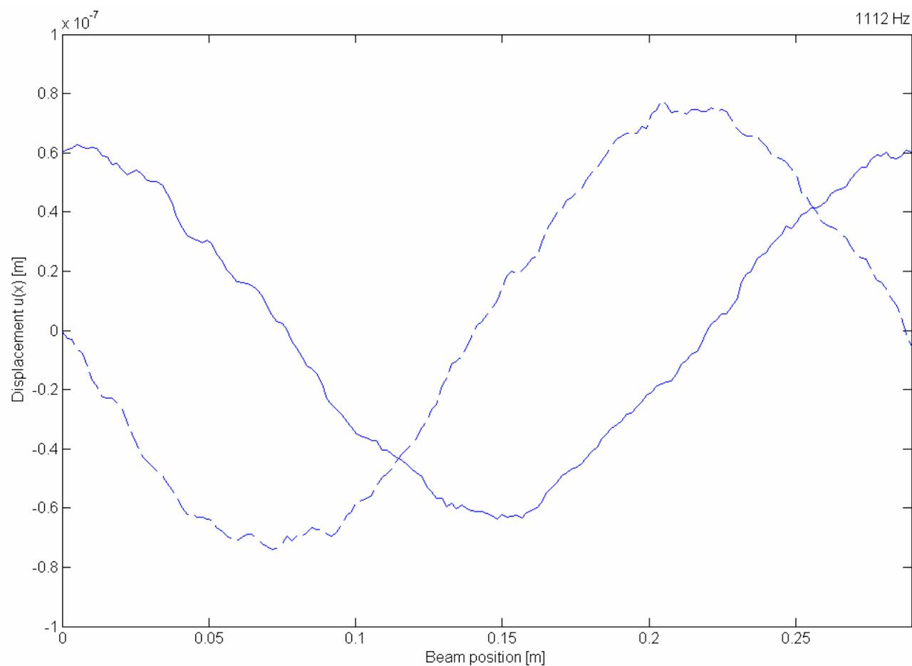
Figure 13. Real part (—) and imaginary part (----) of row 150 from a single cycle of beam displacement at 1112 Hz.
