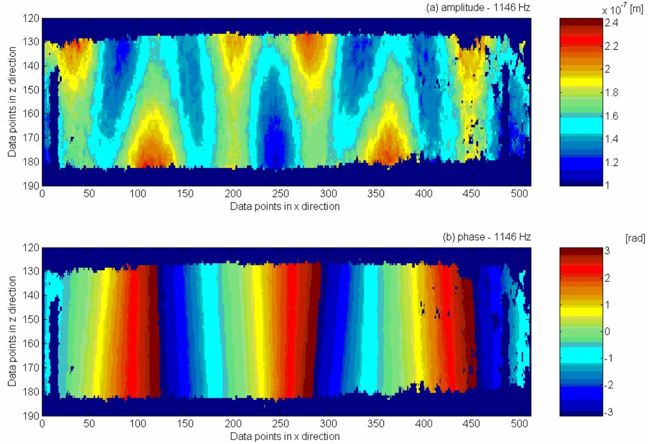
Figure 7. ESPI image of beam displacement excited by a harmonic force at 1146 Hz, (a) amplitude, (b) phase.
