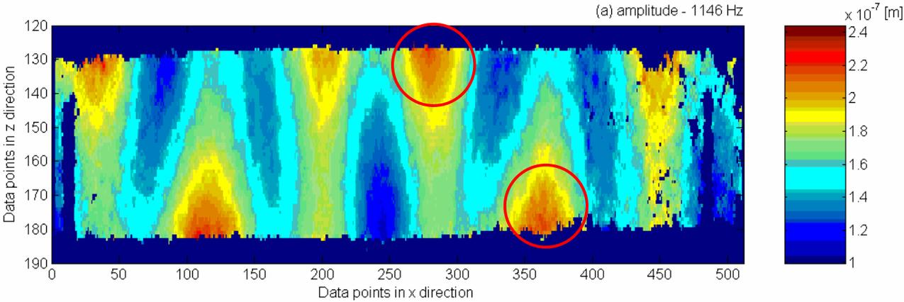
Figure 8. Beam displacement amplitude showing regions of high vibration amplitude due to torsional vibration at 1146 Hz (indicated with circles).
