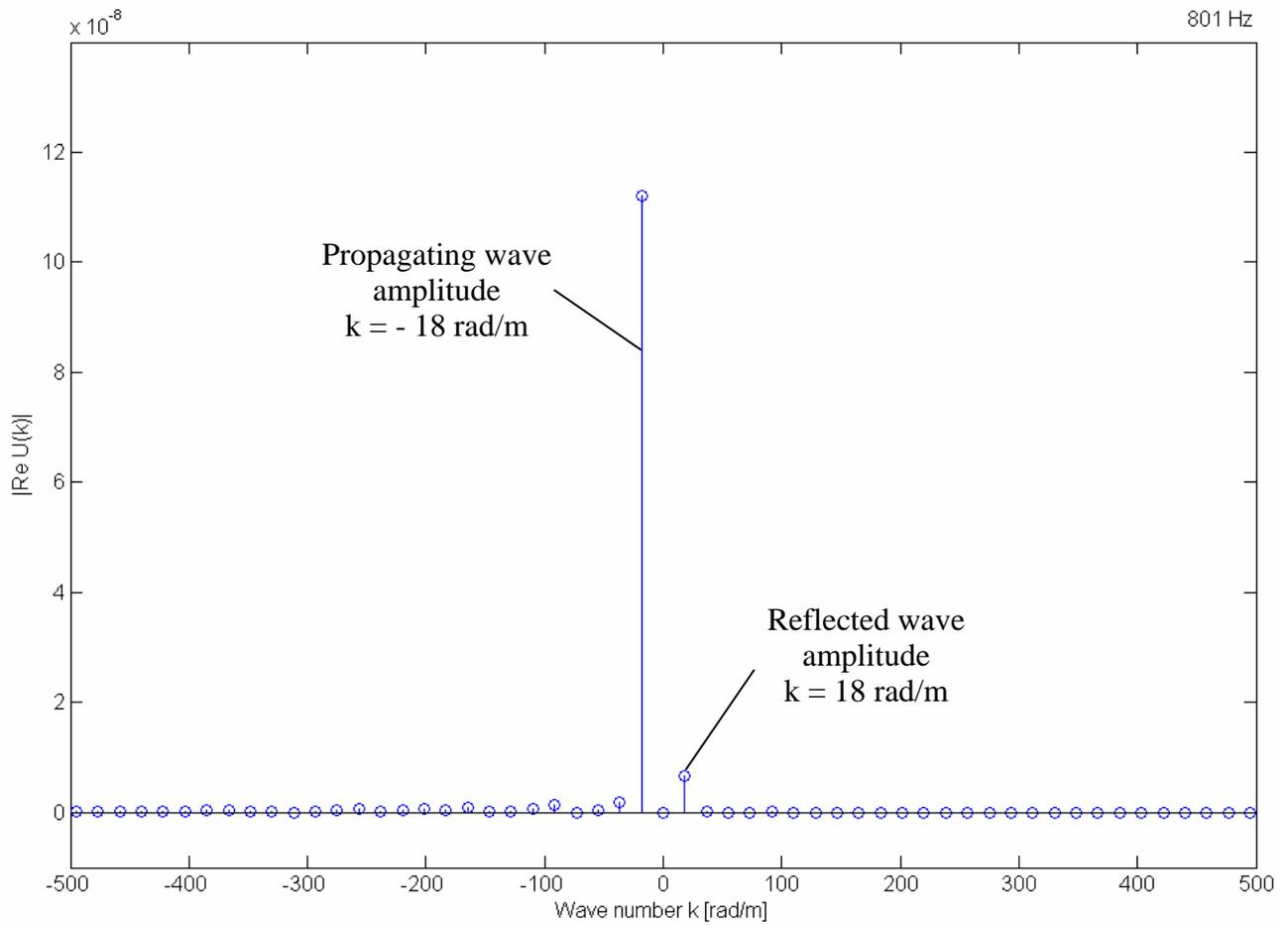
Figure 15. Real part of the wavenumber spectrum of the displacement showing propagating and reflected wave components at 801 Hz.
