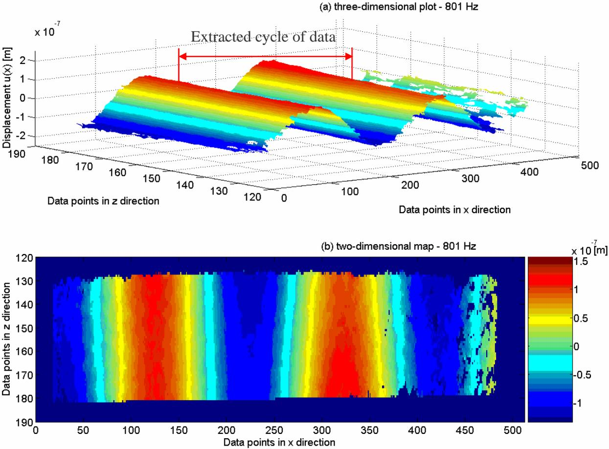
Figure 9. Real part of the beam displacement at 801 Hz showing the single cycle extracted for wavenumber transformation: (a) three-dimensional plot, (b) two-dimensional map.
