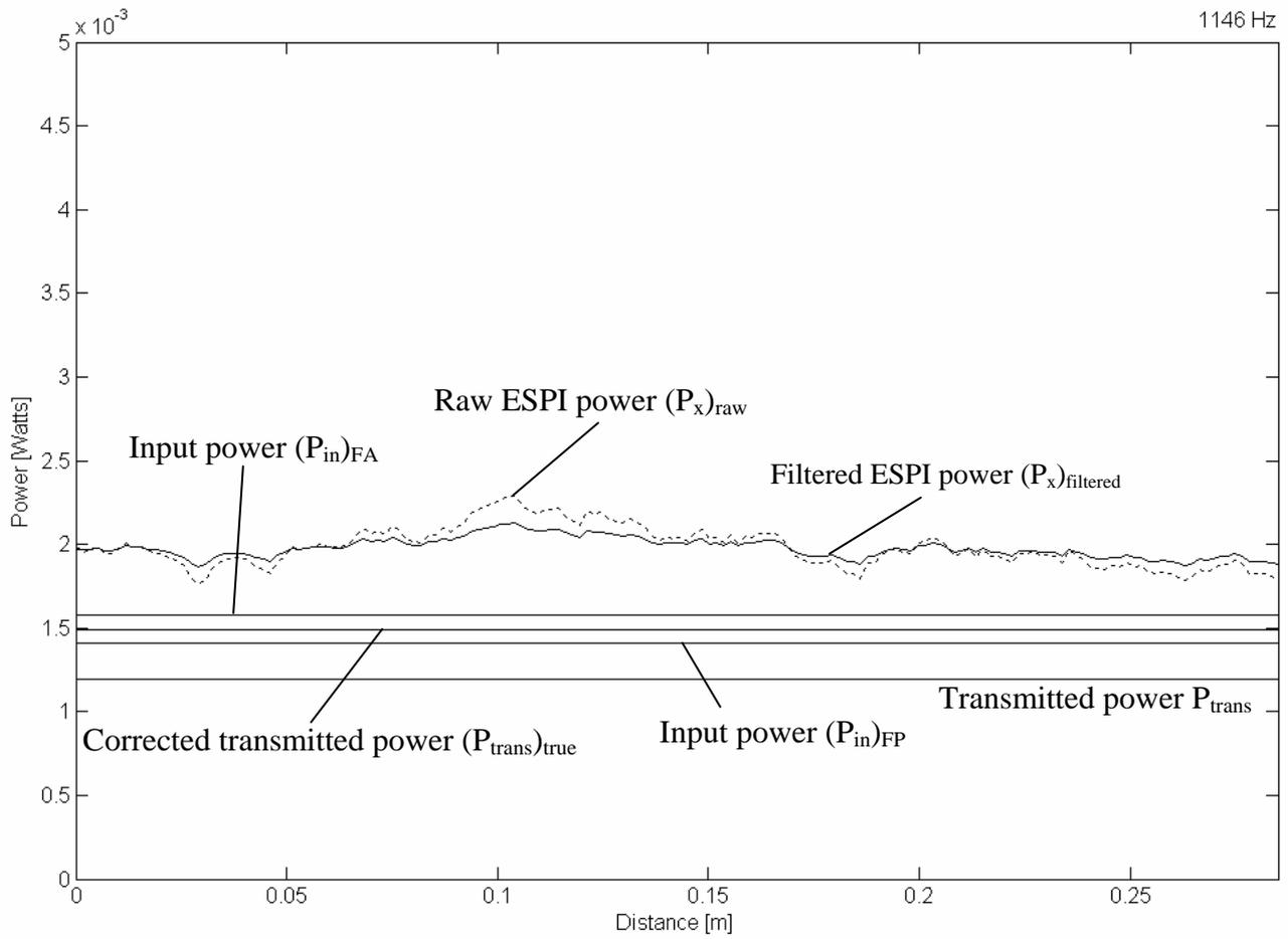
Figure 20. Comparison of measured input power and measured transmitted power against distance along the ESPI window of the experimental beam at 1146 Hz, row 150.
