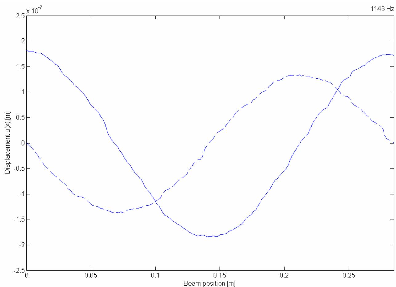
Figure 14. Real part (—) and imaginary part (----) of row 150 from a single cycle of beam displacement at 1146 Hz.
