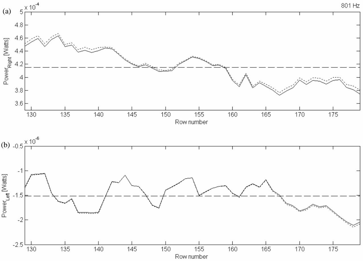
Figure 21. Power flow distribution across the beam width, raw ESPI power (.....), filtered ESPI power (—) and averaged value (----) at 801 Hz: (a) right going wave; (b) left going wave.
