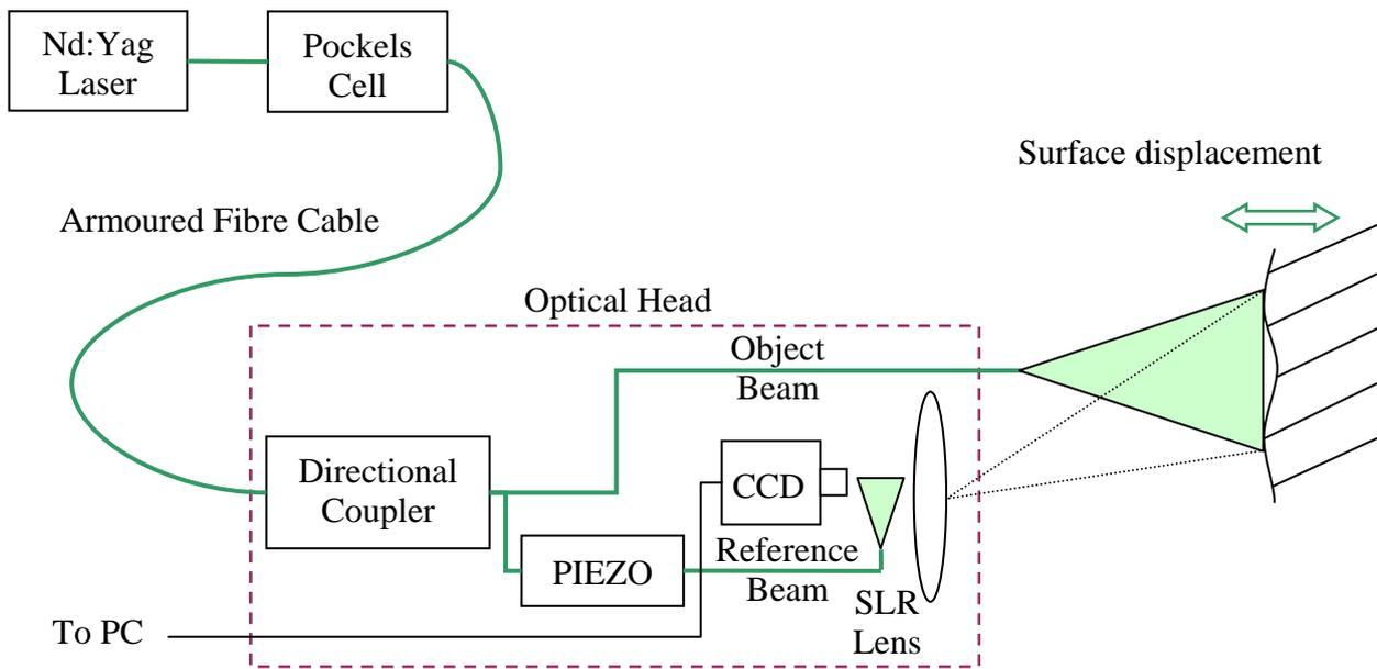
Figure 2. ESPI measurement system.
