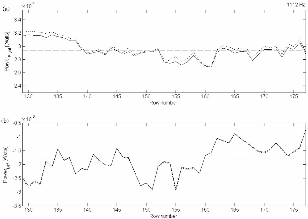
Figure 22. Power flow distribution across the beam width, raw ESPI power (.....), filtered ESPI power (—) and averaged value (----) at 1112 Hz: (a) right going wave; (b) left going wave.
