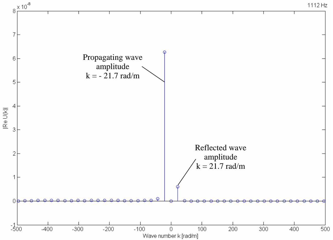
Figure 16. Real part of the wavenumber spectrum of the displacement showing propagating and reflected wave components at 1112 Hz.
