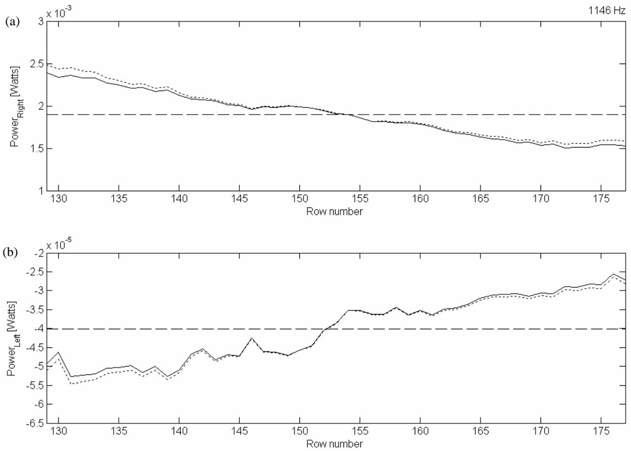
Figure 23. Power flow distribution across the beam width, raw ESPI power (.....), filtered ESPI power (—) and averaged value (----) at 1146 Hz: (a) right going wave; (b) left going wave.
