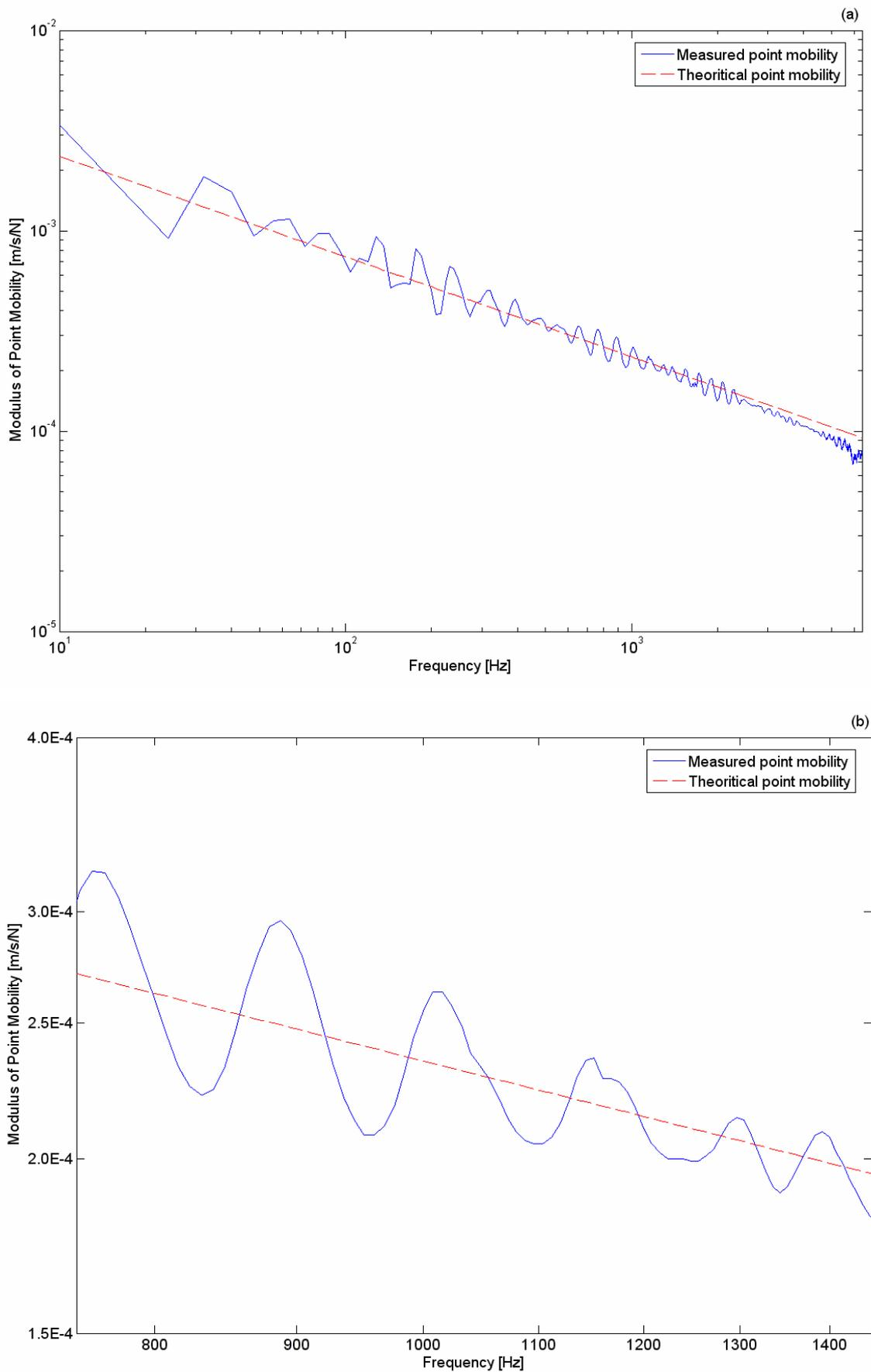
Figure 4. Driving Point mobility of the experimental "infinite" beam, measured (—) and theoretical (-----), (a) 10-10kHz, (b) 750-1450 Hz.
