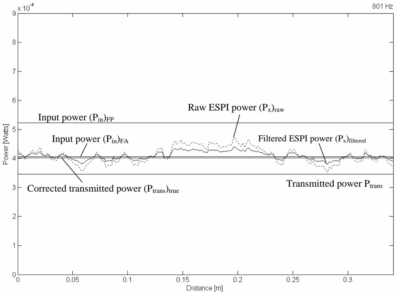
Figure 18. Comparison of measured input power and measured transmitted power against distance along the ESPI window of the experimental beam at 801 Hz, row 150.
