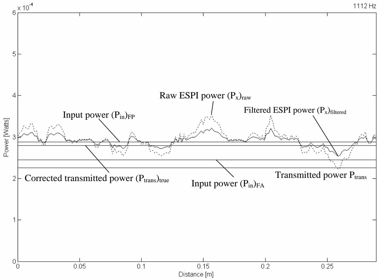
Figure 19. Comparison of measured input power and measured transmitted power against distance along the ESPI window of the experimental beam at 1112 Hz, row 150.
