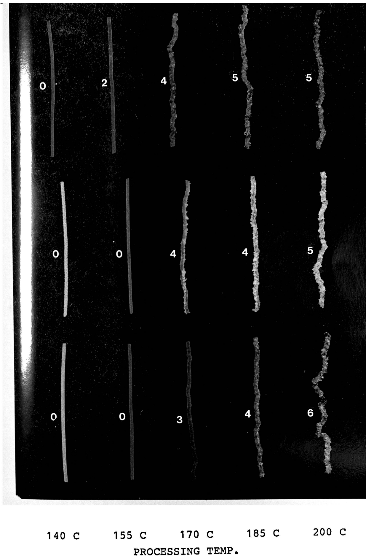
Fig.5.12 Variation of extrudate distortion with processing temperature (samples extruded at 140 C).
