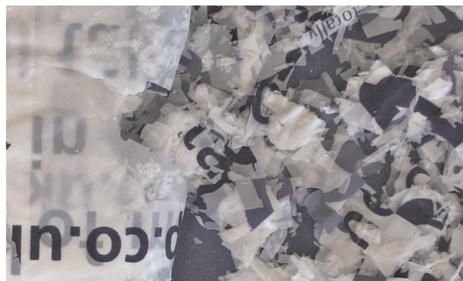
**Figure 1.** Illustrating degradation of an oxo-degradable carrier bag
