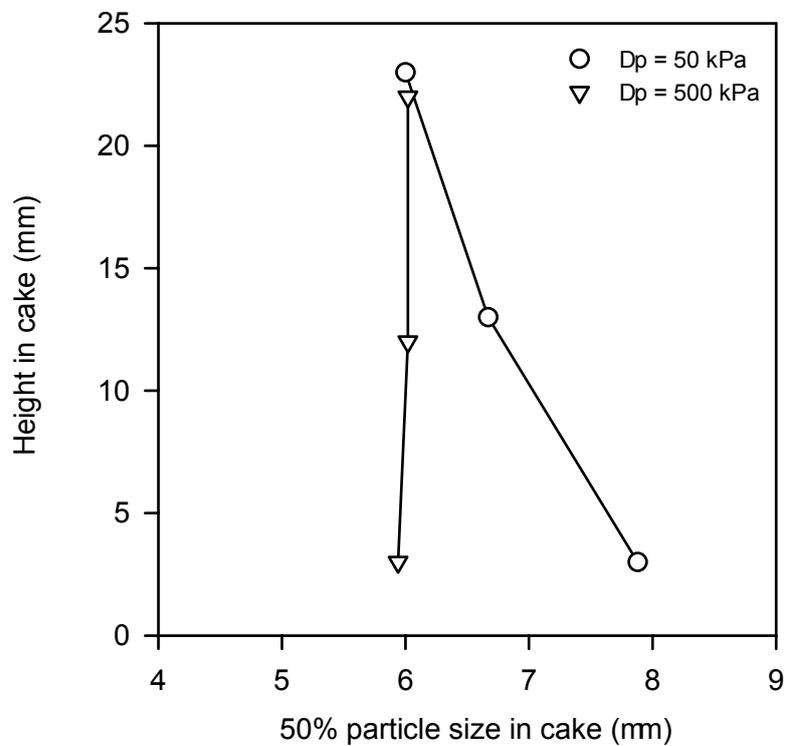
Figure 10: The effects of filtration pressure on the measured particle size in a filter cake; mix 2.
