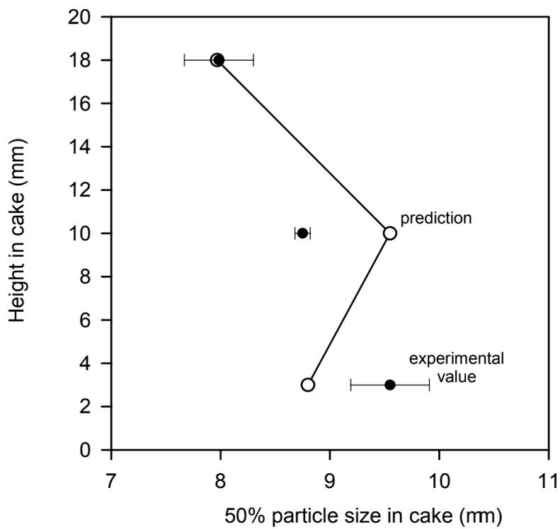
Figure 8: Experimental and theoretical particle sizes in a filter cake; mix 1,  $\Delta p = 100$  kPa.
