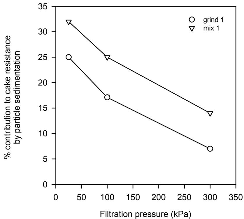
Figure 6: Predicted contributions of particle sedimentation to cake resistance as a function of filtration pressure.
