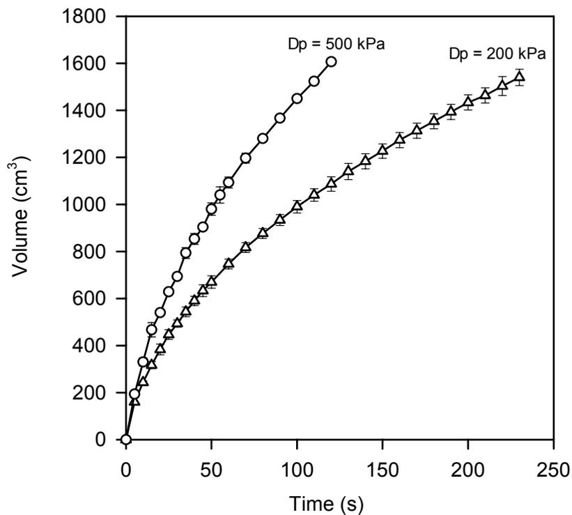
Figure 2: Typical variations between repeat filtration tests; unground 2.
