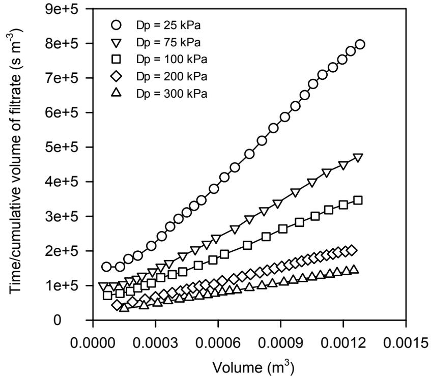
Figure 3: Sequential variation of experimental data with filtration pressure; grind 1.
