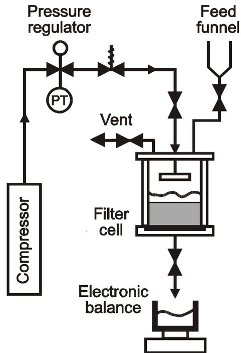
Figure 1: Schematic of the dead-end filtration apparatus.
