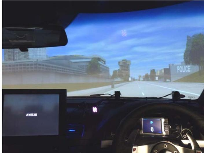
**Figure 1** Location of the visual display in the simulator vehicle
