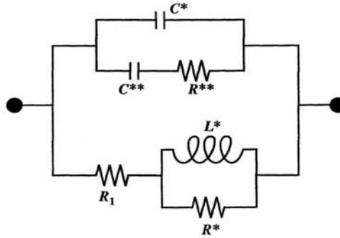
**Fig. 2.** The two-terminal equivalent network of a three-terminal electrochemical cell. Note the series/parallel arrangement of elements, which greatly simplifies the network analysis. Asterisks (\*) indicate experimental artefacts.
