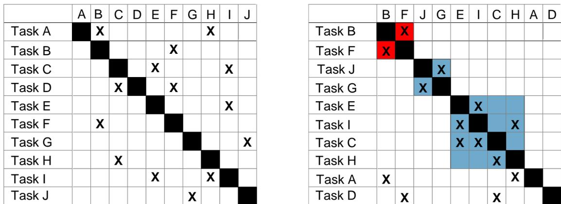
Figure 4. Example of DSM Analysis before and after partitioning
