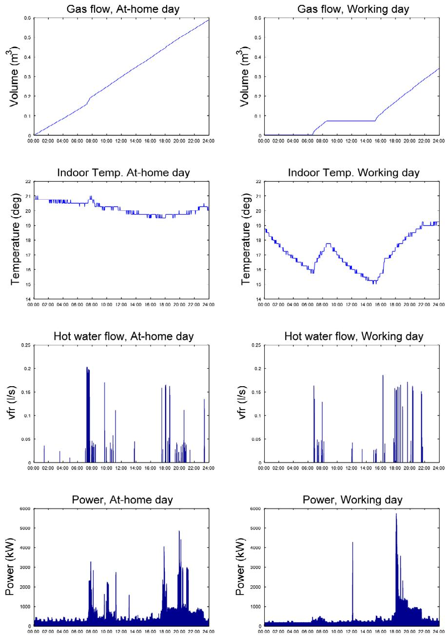
Figure 1: Energy consumption profiles for a working day and a weekend day.
