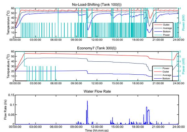
Figure 2: Tank temperature oscillations and power consumption for two cases: tank 100(l) and *No Load Shifting* (top plot); tank 300(l) and *Economy7* (middle plot) as considering the hot water usage profile (bottom plot).
