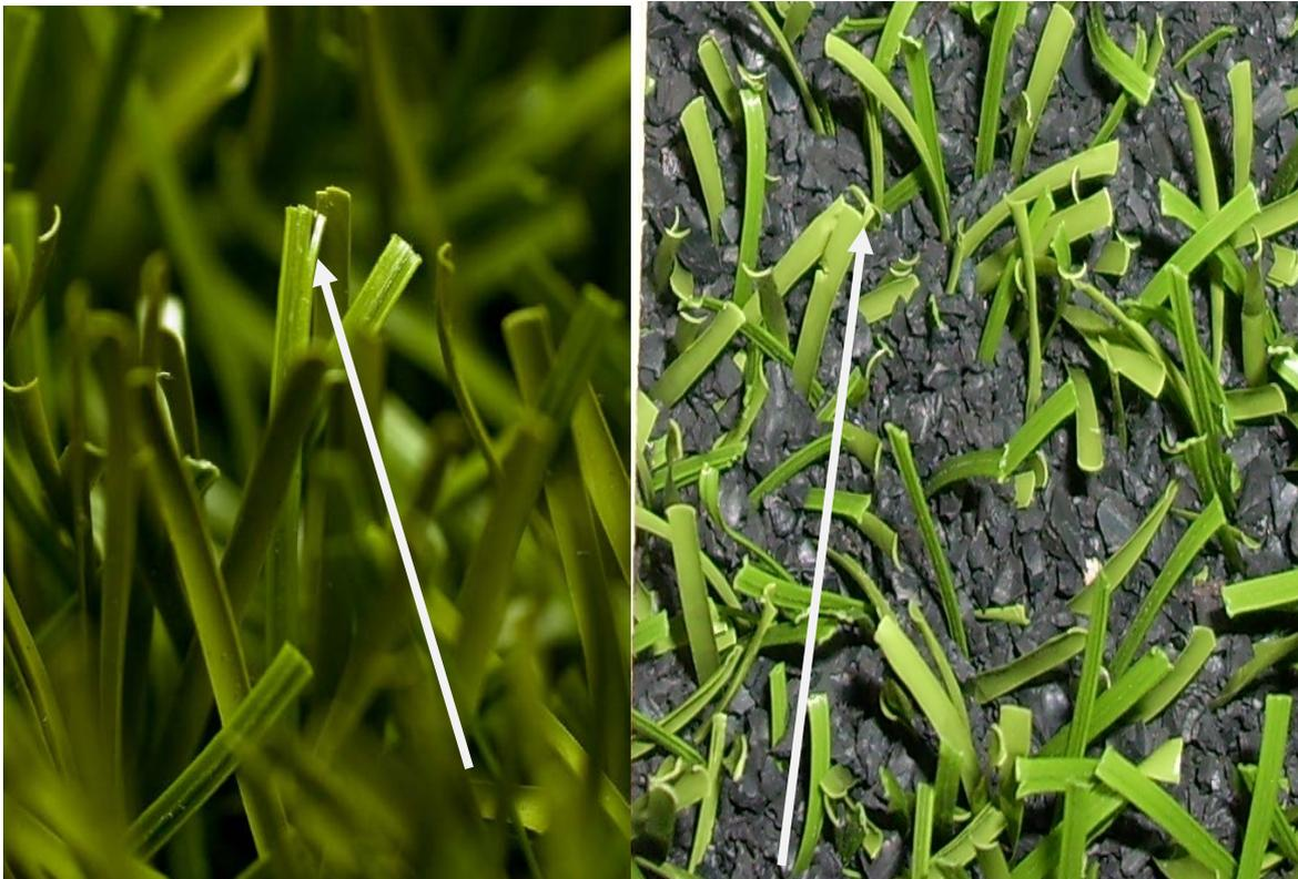
Plate 4 – Examples of fibre a) splits and b) breaks from brushing
