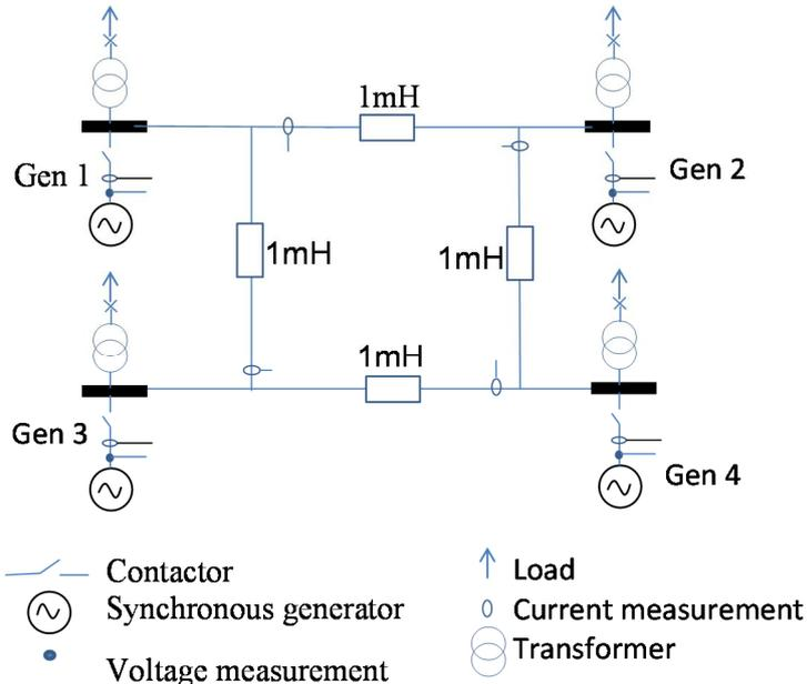
Fig. 1 . A schematic of the micro-grid system.
