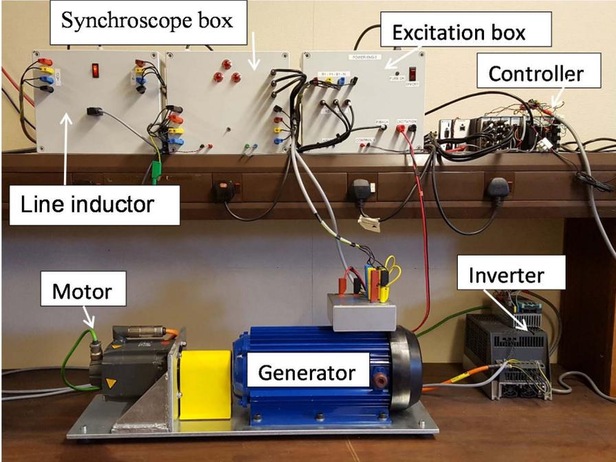
Fig. 2 Hardware components for each micro grid generator
