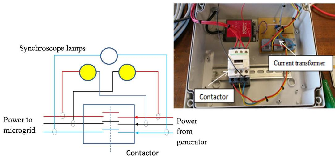
Fig. 5 Synchroscope box
