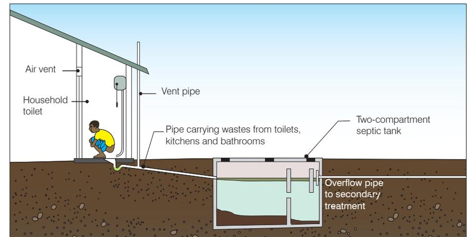
**Figure 1.** Wastewater treatment using a septic tank
