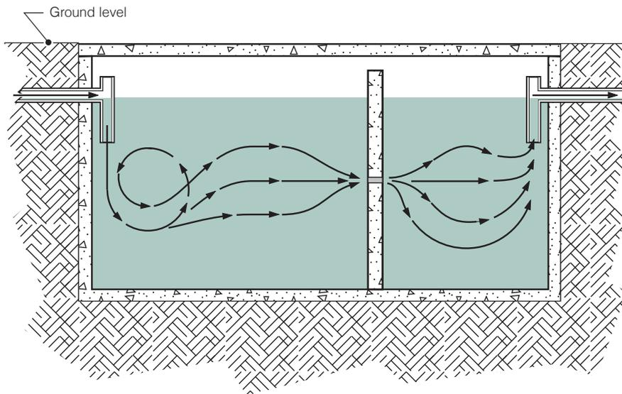
Large tank – turbulence takes up a much smaller proportion of the first tank
