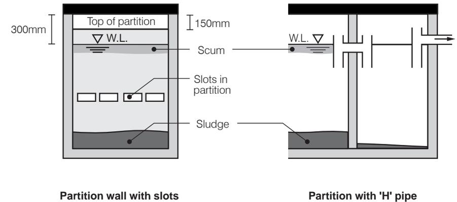
**Figure 10.** Options for flow through tank partitions
