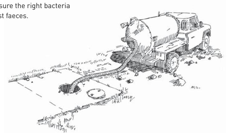
**Figure 12.** Sludge removal
