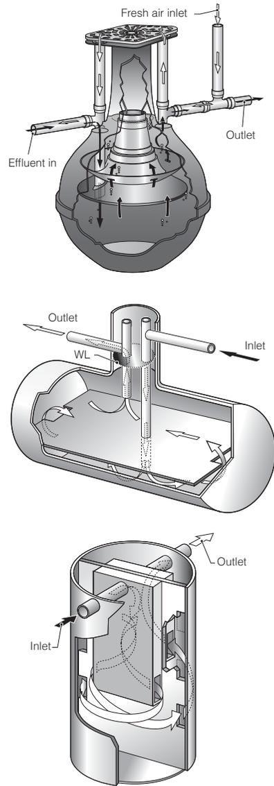
**Figure 11.** Examples of pre-fabricated septic tanks
