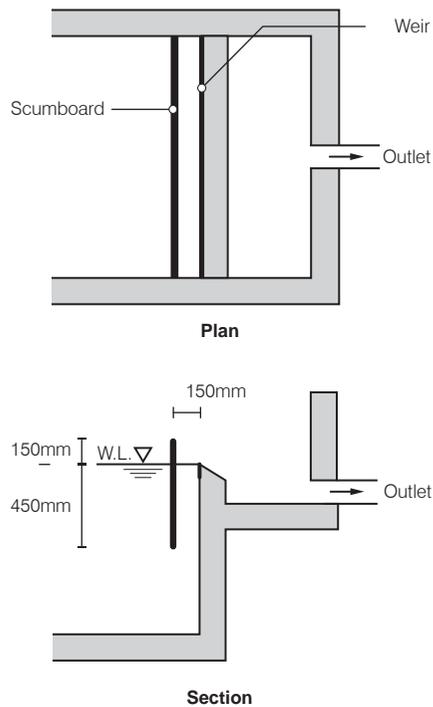
Figure 9. Tank outlet using overflow weir
