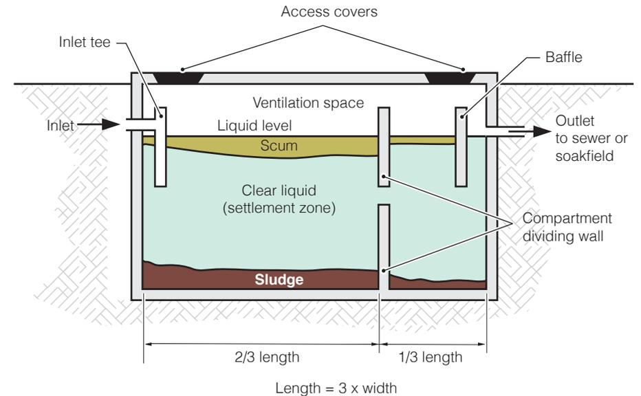
**Figure 5.** Treatment process in a septic tank
