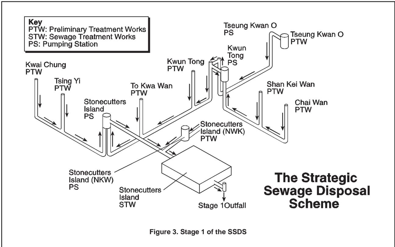
Figure 3. Stage 1 of the SSDS
