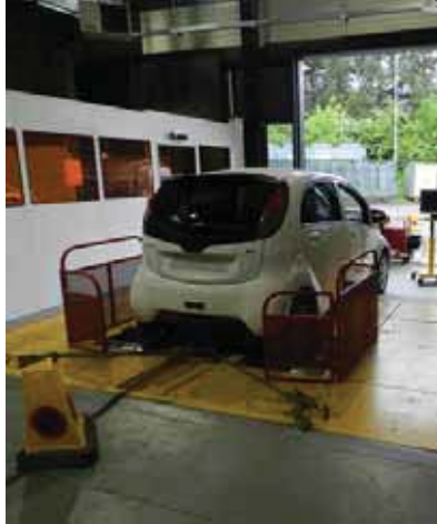
Fig. 3-A. Vehicle under test mounted on the chassis dynamometer (roller bench)
