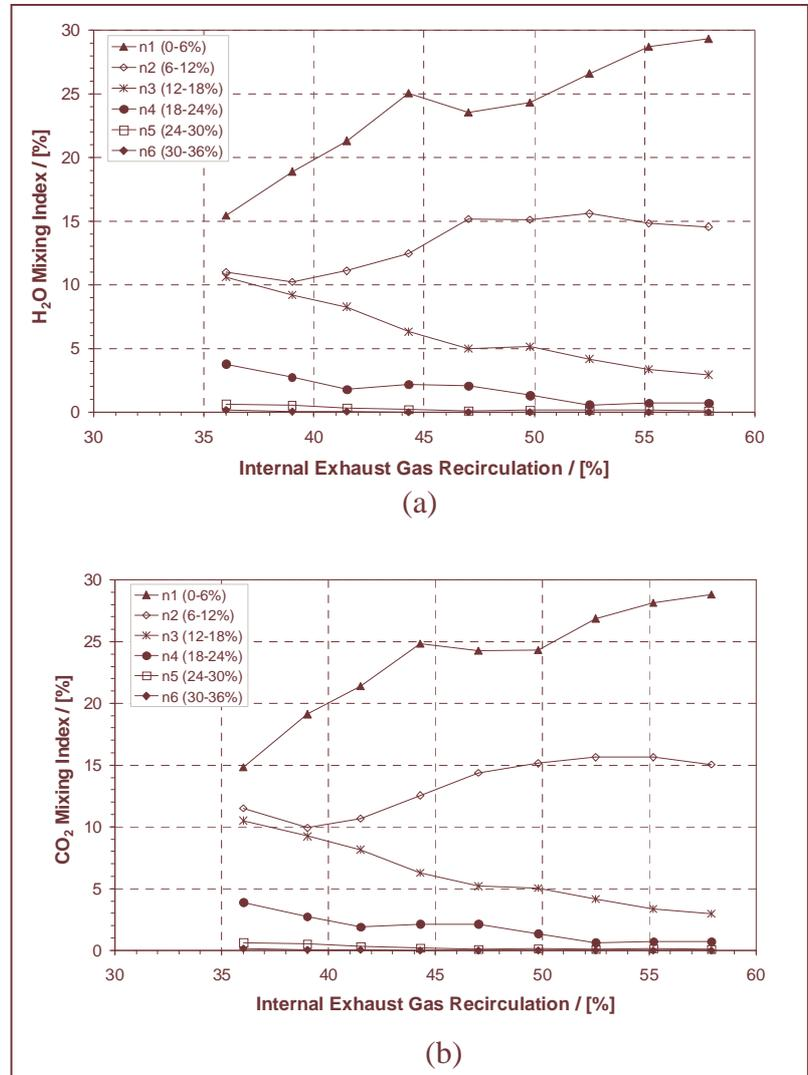
Fig 7: Mixing index plots vs. IEGR (a) H<sub>2</sub>O index (b) CO<sub>2</sub> index
