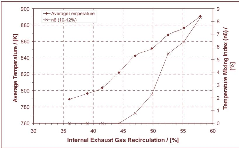
Fig 5: In cylinder average temperature and temperature mixing index vs. IEGR at 720 crank angle
