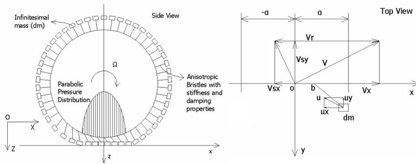
Fig. 1. Side and Top view of the tyre model, depicting an arbitrary position of infinitesimal mass.
