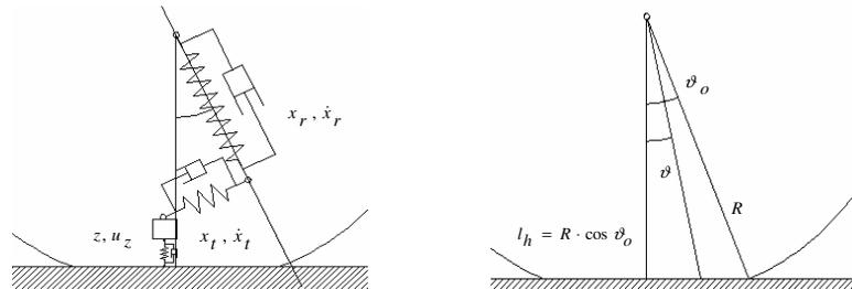
Fig. 3. The modified tyre model and some important dimensions
