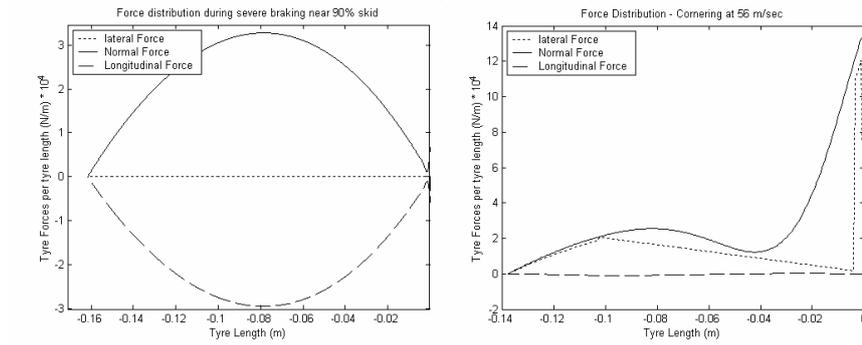
Fig. 7. Normal pressure distribution for hard acceleration and high speed cornering
