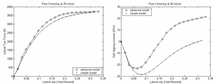
Fig. 4. Cornering force and self-aligning moment
