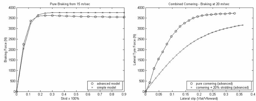
Fig. 5. Braking Force and lateral force during combined cornering - braking
