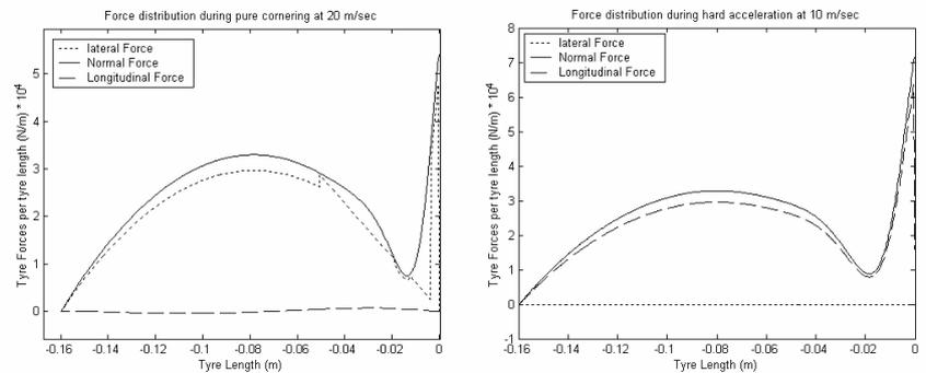
Fig. 6. Normal pressure distribution for purely cornering conditions
