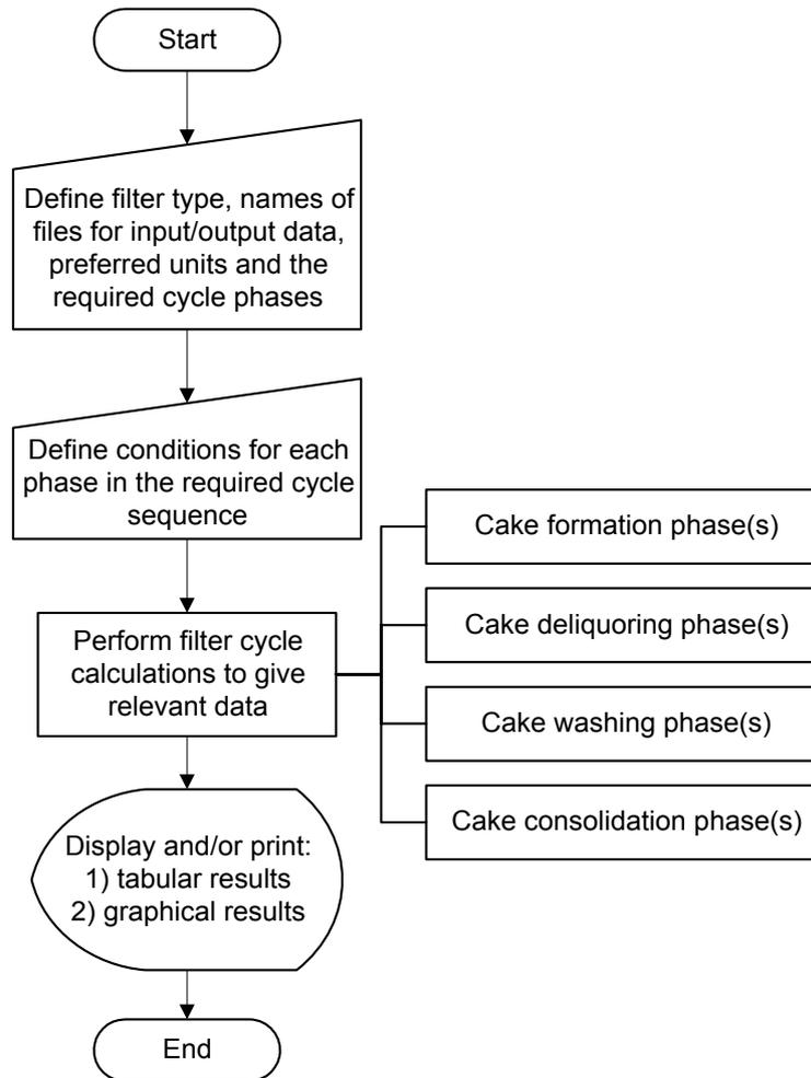
Figure 5: Basic flowsheet for modular filter simulations.
