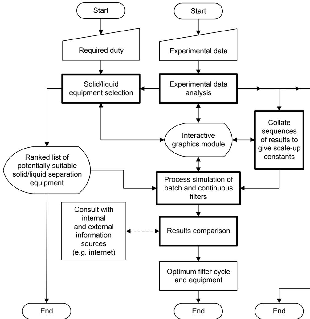
Figure 7: Outline schematic of the integration of equipment selection, scale-up and process simulation.
