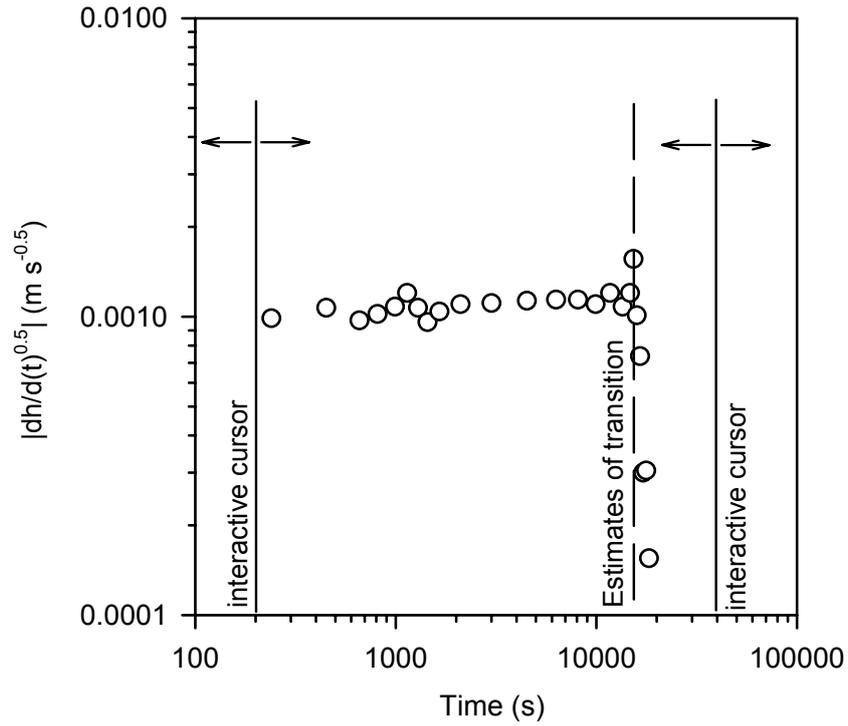
Figure 3: Estimating the filtration to cake consolidation transition via software<sup>5</sup>.
