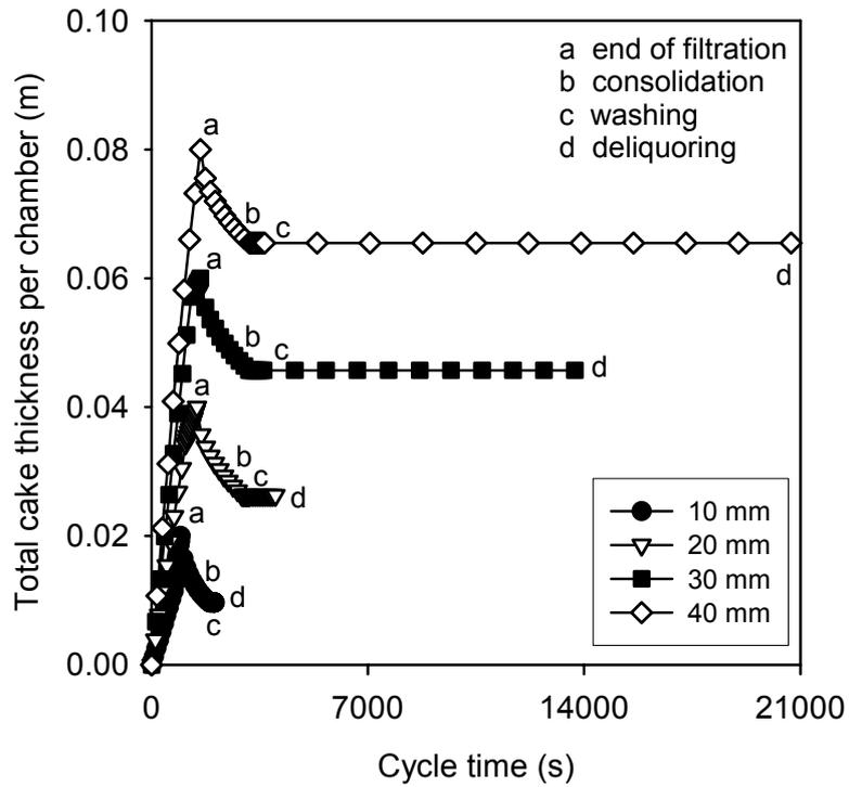
Figure 6: Sample results from a diaphragm press simulation.
