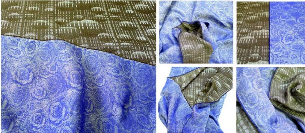
Figure 8. Single color double-cloth fabrication in natural shading effect.
