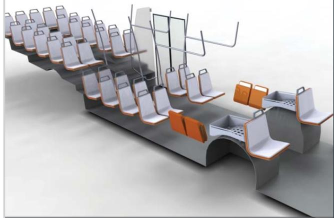
Modular components used to fit out the interior of a conventional rigid route bus to an existing customer specification – number of seats and layout thereof
