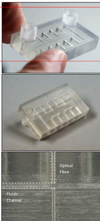
Figure 8. 3D serpentine mixing device used in optimisation (a) top (b) bottom (c) close up of monitoring region showing fibers intersecting fluidic channel
