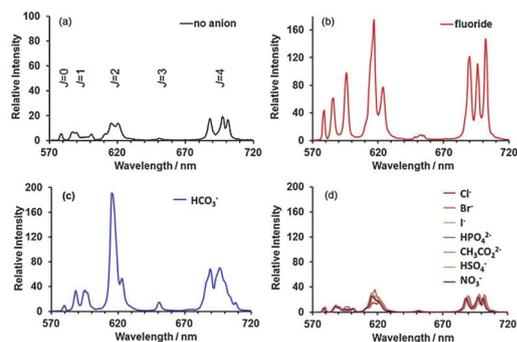
Fig. 2 Comparison of the emission spectrum of (a)  $[\text{Eu.L}^1]^+$  with the limiting emission spectra of  $[\text{Eu.L}^1]^+$  in the presence of: (b) 2 mM fluoride; (c) 2 mM  $\text{HCO}_3^-$ ; and (d) 2 mM  $\text{Cl}^-$ ,  $\text{Br}^-$ ,  $\text{I}^-$ ,  $\text{HPO}_4^{2-}$ ,  $\text{CH}_3\text{CO}_2^-$ ,  $\text{HSO}_4^-$ ,  $\text{NO}_3^-$  (sodium salts). Conditions:  $\text{H}_2\text{O}$  (25 mM HEPES, pH 7.4),  $\lambda_{\text{exc}} = 332$  nm, 298 K.
