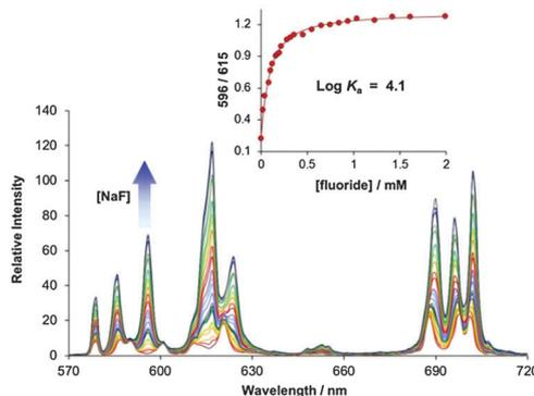
Fig. 3 Change in emission spectra of  $[\text{Eu.L}^1]^+$  (20  $\mu\text{M}$ ) as a function of added NaF. Conditions:  $\text{H}_2\text{O}$  (25 mM MES, pH 6.0),  $\lambda_{\text{exc}} = 332$  nm, 298 K. The inset shows the fit to the experimental data, for  $\log K_a = 4.1$  ( $\pm 0.1$ ).
