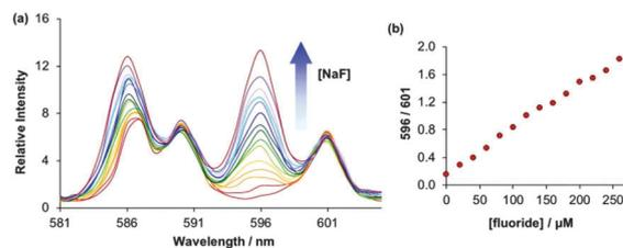
Fig. 6 (a) Ratiometric change in emission spectral form of  $[\text{Eu.L}^1]^+$  (20 μM) within the  $\Delta J = 1$  manifold (580–605 nm), as a function of added NaF (0–260 μM). (b) Linear increase in the emission intensity ratio, 596/601 nm, in the range relevant to water fluoridation. Conditions: H<sub>2</sub>O (25 mM MES, pH 6.0),  $\lambda_{\text{exc}} = 332$  nm, 25 °C.
