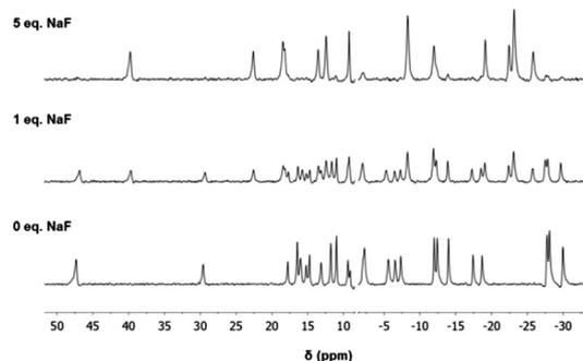
Fig. 5 <sup>1</sup>H NMR spectra of  $[\text{Eu.L}^1]^+$  (2.4 mM) upon addition of NaF (0–5 eq.). Measured in D<sub>2</sub>O (pD 6.4, 298 K).
