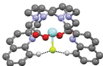
Fig. 4 An optimised structure of  $[\text{Eu.L}^2]^+$  with a coordinated fluoride ion, stabilised by two short C-H...F<sup>-</sup> contacts (avg. C-H...F<sup>-</sup> distance is 2.81 Å, avg. C-H...F<sup>-</sup> angle is 141°). The model geometry was optimised at B3LYP/3-21G\* (Gaussian 09 package) using the crystal structure of an Eu complex reported in ref. 14 as a starting point.
