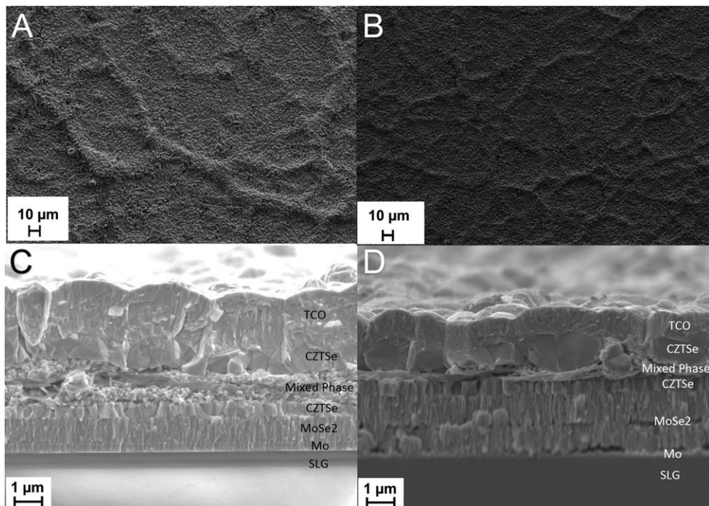
**Fig. 3.** A) SEM surface image after a 20 min selenisation (2 k× magnification). B) SEM surface image after a 50 min selenisation (1 k× magnification). C) SEM cross-sectional image after a 20 min selenisation. D) SEM cross-sectional image after a 50 min selenisation.
