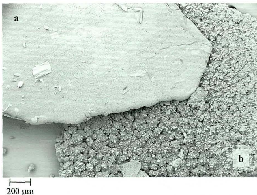
Figure 83 – SEM image of two (SN)_x plates showing both (a) ‘smooth’ and (b) ‘growth’ surface types.
