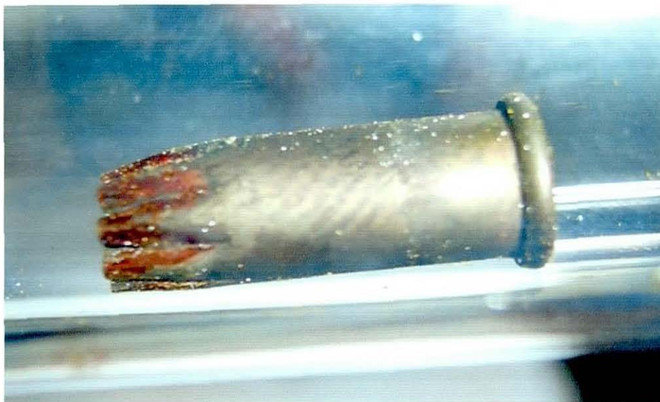
Figure 45 – (SN)_x enhanced fingerprint on a spent cartridge shell; photograph taken in situ through the glass side-arm.
