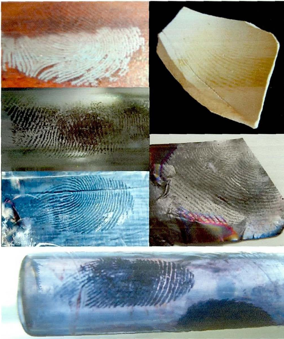
Figure 41 – The induced growth of (SN)_x over latent fingermark residues on various sample surfaces (Clockwise from top left: wood, ceramic pottery, aluminium foil, clingfilm, adhesive tape, glass).
