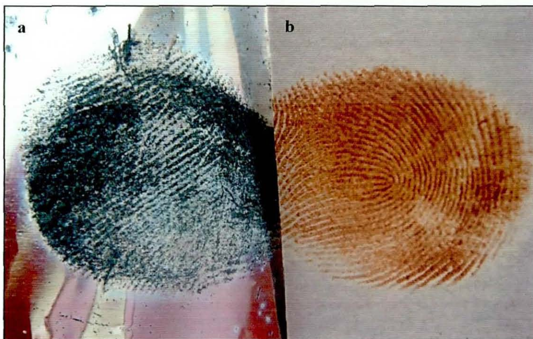
Figure 102 – Latent fingerprints on (a) aluminium foil and (b) paper, enhanced following exposure to \text{NSCl} vapour.
