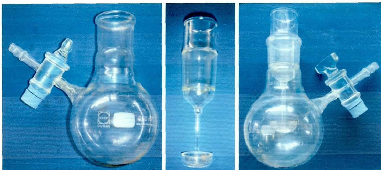
Figure 99 – The custom apparatus used during in situ NSCl reactions with various zeolite media.
