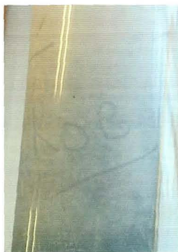
Figure 57 – A written impression, three sheets below the original text, detected and enhanced by (SN)_x .
