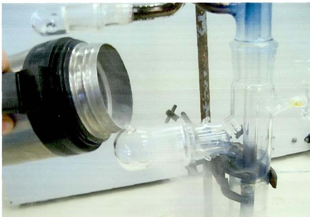
Figure 85 – Photograph showing the method used to isolate single crystals of S_2N_2 used for XRD.
