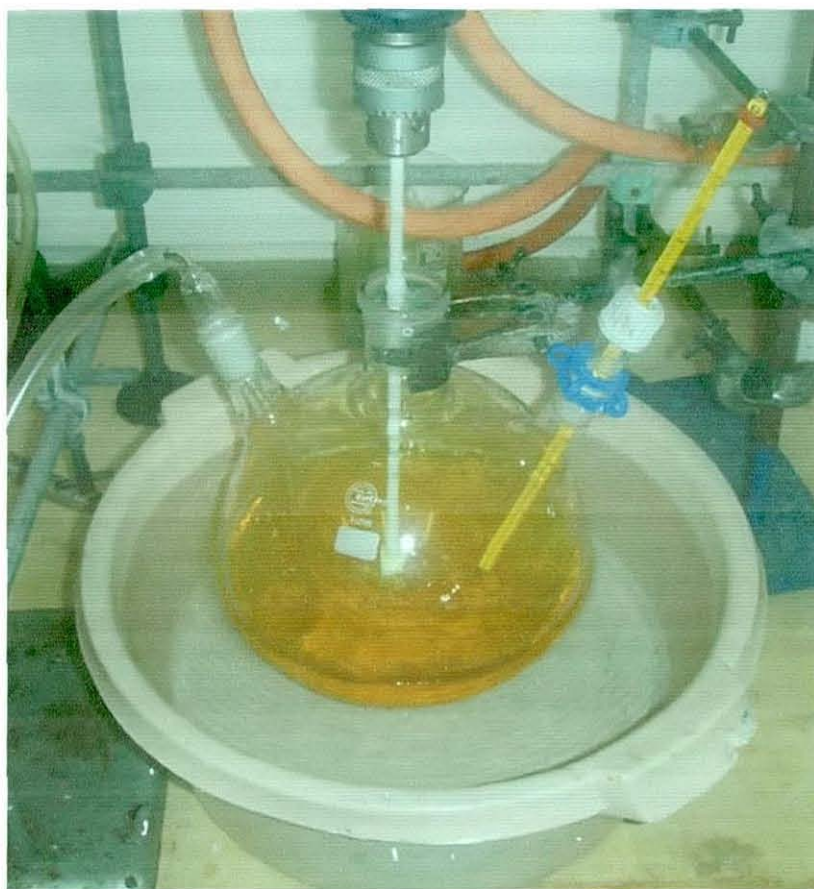
Figure 17 – The apparatus used to prepare crude S_4N_4 .
