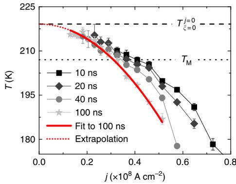
**Fig. 3** Temperature of  $H_x$  independence at various current densities.  $T$  at which  $\xi = 0$  versus current density  $j$  for 10 ns, 20 ns, 40 ns and 100 ns long voltage pulses. Fit to data of 100 ns long pulses used to obtain temperature  $T_{\xi=0}^{j=0}$  at which  $\xi = 0$  in the limit of no heating by extrapolation of fit. Error bars reflect errors in  $T_{\xi=0}^{j=0}$  obtained by fits to data (Fig. 2c and Supplementary Fig. 3-5)
