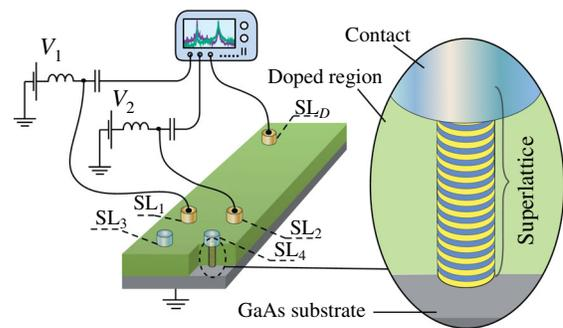
FIG. 1. The design of the experimental setup. Generators  $SL_{1,2}$  and the detector  $SL_D$  (gold) are involved in our experiments.  $SL_{3,4}$  (blue) are additional devices used in our numerical simulations.
