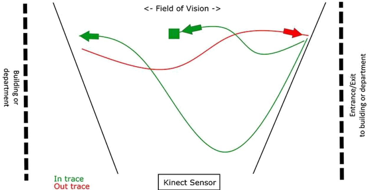
**Figure 2: Diagrammatic illustration of SmartCounter3D**
