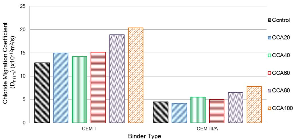
Figure 6: Chloride migration coefficients at 28 days
