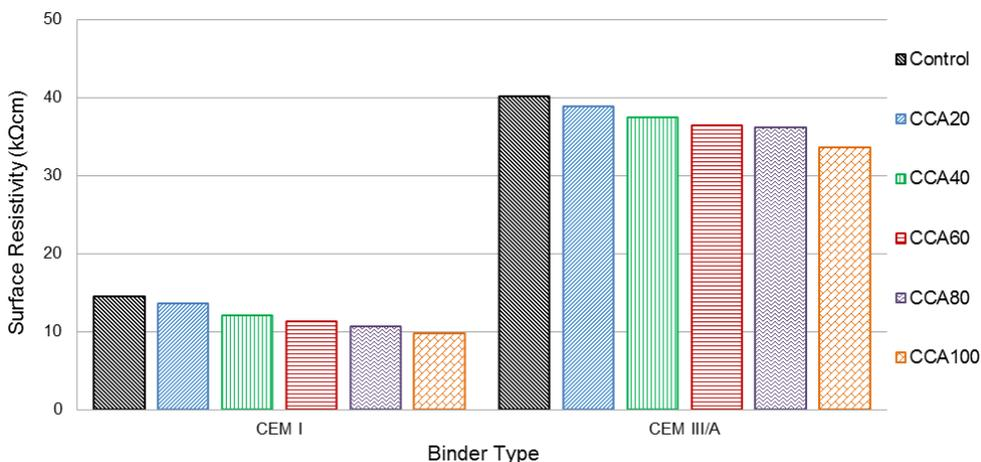
Figure 4: Concrete surface resistivity at 28 days
