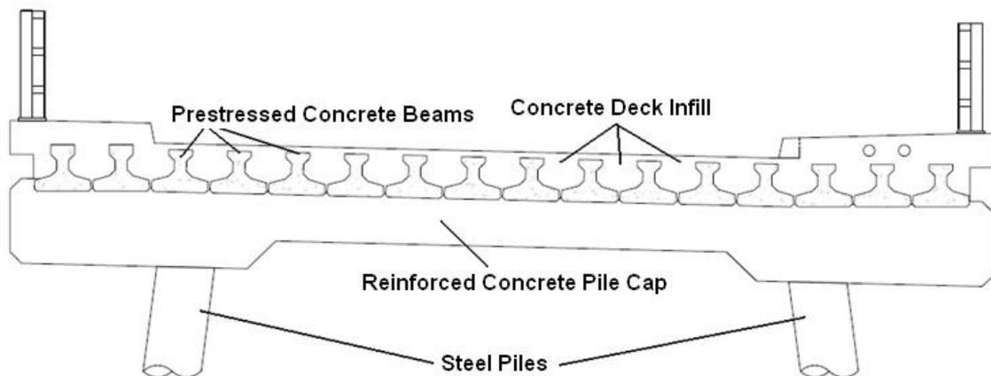
Figure 2: Typical structural cross section of the bridge
