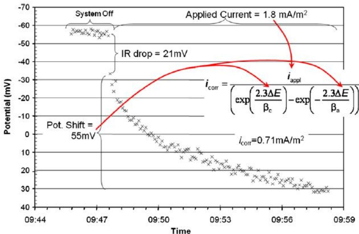
Figure 7: Example corrosion current density calculation (Christodoulou et al. 2010)
