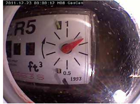
Figure 1: A typical rotating dial on an older UK gas meter.
