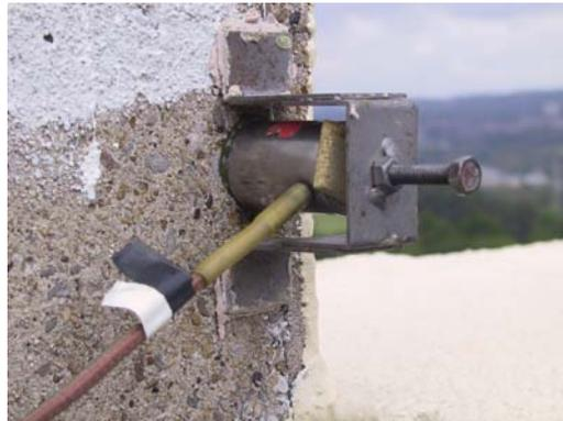
**Figure 1** Transducer Mounting
